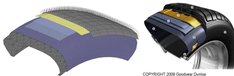
Figure 3: Functional component layers of the tire
