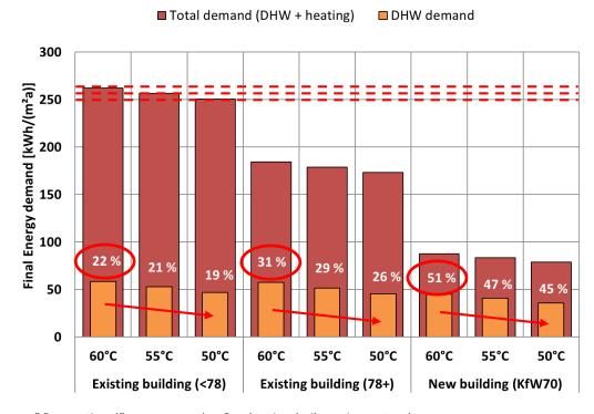
"Conventional" energy supply: Condensing boiler using natural gas
