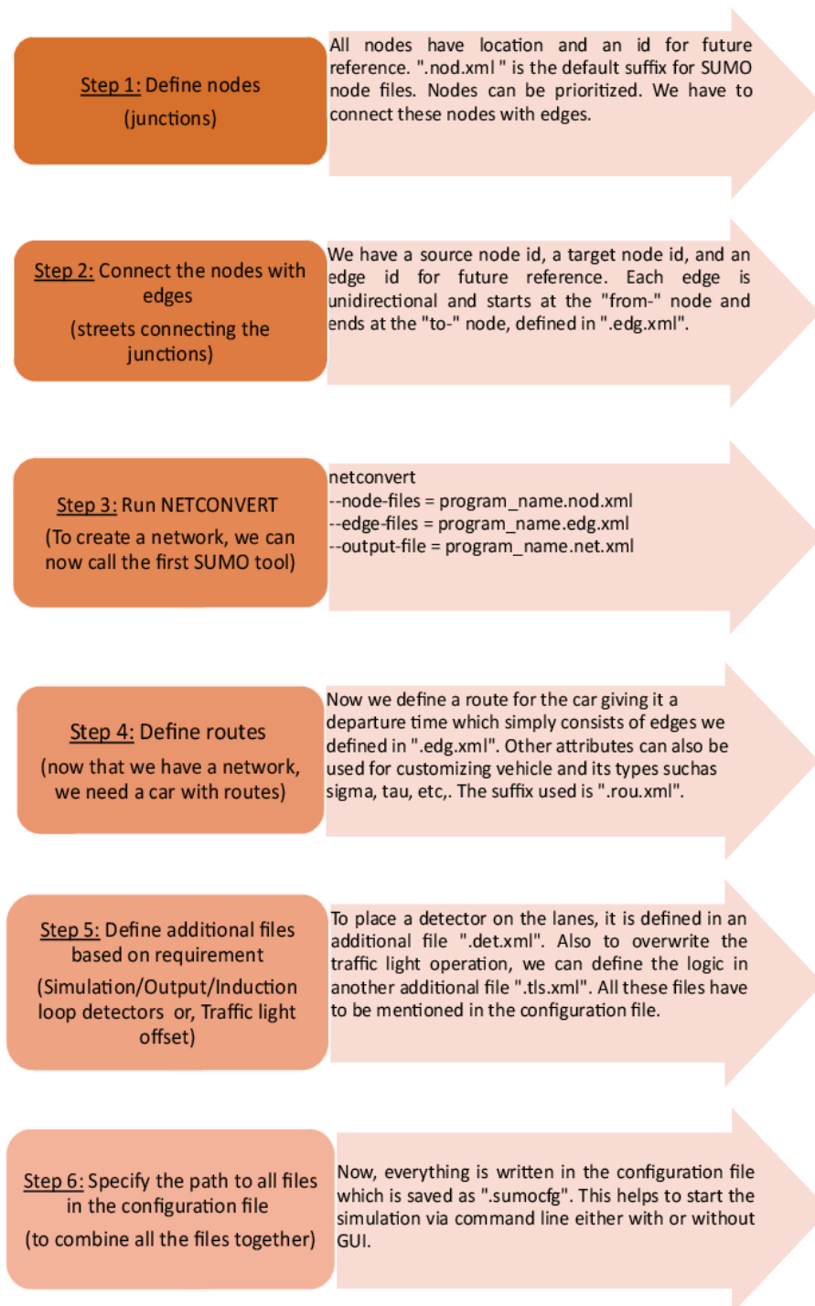
FIGURE 3.2: Process chart showing steps involved in building a scenario using XML for simulation using SUMO simulator
