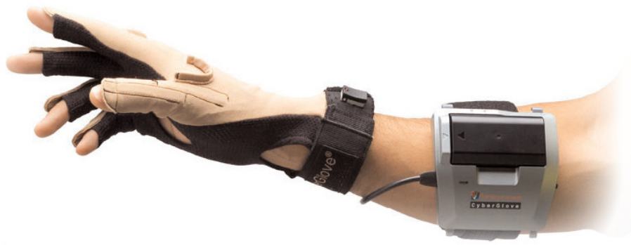
Figure 2.6: A data glove with 18 sensors, which is capable of estimating the bending and the abduction angle of all fingers (Courtesy of Immersion Corporation, www.immersion.com ).
