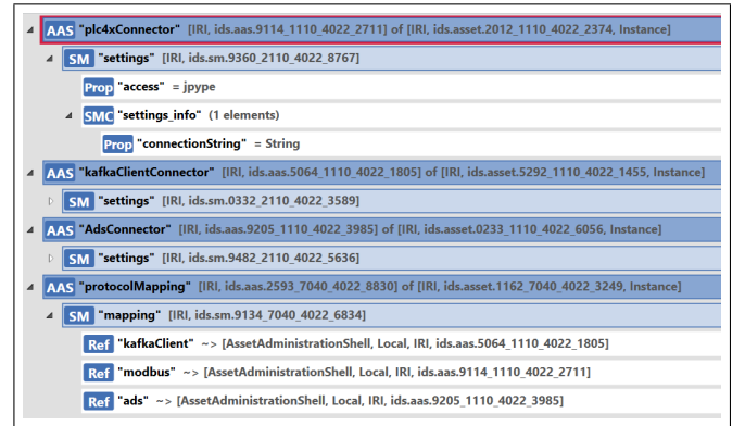
Fig. 5. Screenshot of the .AASX file with the connector information for the modular production use case.
