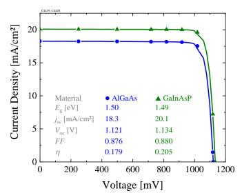
Fig. 5. Current-voltage characteristics of an  $Al_{0.06}Ga_{0.94}As$  (blue) and a  $Ga_{0.90}In_{0.10}As_{0.80}P_{0.20}$  (green) rear-heterojunction solar cell with the same absorber layer thickness of 2  $\mu$ m.
