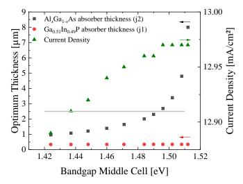
Fig. 7. Required thickness of middle cell absorber layer as a function of the band gap to achieve current matching conditions in a III-V//Si triple-junction solar cell. The grey line indicates a reference value for the diffusion length in p-AlGaAs as measured by cathodoluminescence.
