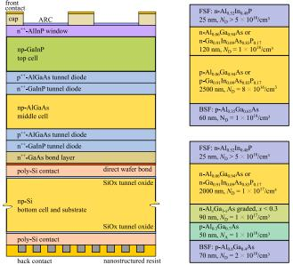
Fig. 1. Left: The III-V//Si triple-junction solar cell layer stack with an efficiency of 34.1 % under AM1.5g. The currently used middle cell consists of a mostly p-type AlGaAs absorber in a homojunction design. Right: Structures of the homo-junction (top) and rear-heterojunction (bottom) component cells that are examined in this work.
