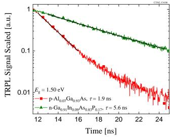
Fig. 6. Comparison of the signal decay transients from TRPL measurements of  $p-Al_{0.07}Ga_{0.93}As$  (red, squares) and  $n-Ga_{0.91}In_{0.09}As_{0.83}P_{0.17}$  (green, triangles) at the same band gap of 1.50 eV. In black the monoexponential fits that were used to extract the minority carrier lifetimes are shown. The non-monoexponential tail at low signal intensities is caused by parasitic luminescence from within the setup and not sample related.
