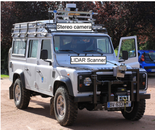
Fig. 1. The experimental platform used in this research provided by the partner IRSTEA and used for field validation in the QUAD-AV project.
