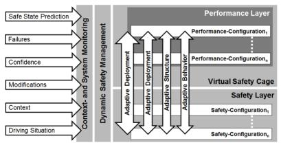
Fig. 1. Basic Concept of Fail-Operational Architectures
