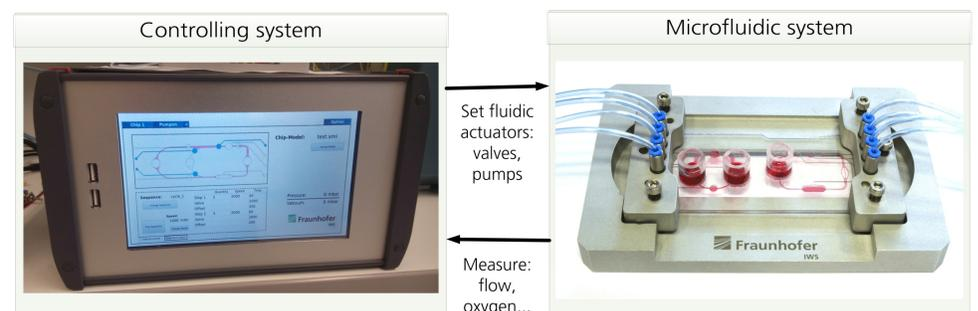
**FIGURE 1:** Cell cultivating device consisting of a microfluidic system and a controlling system which sets fluidic actuators and measures oxygen content. A mathematic model of the fluidic can be implemented.
