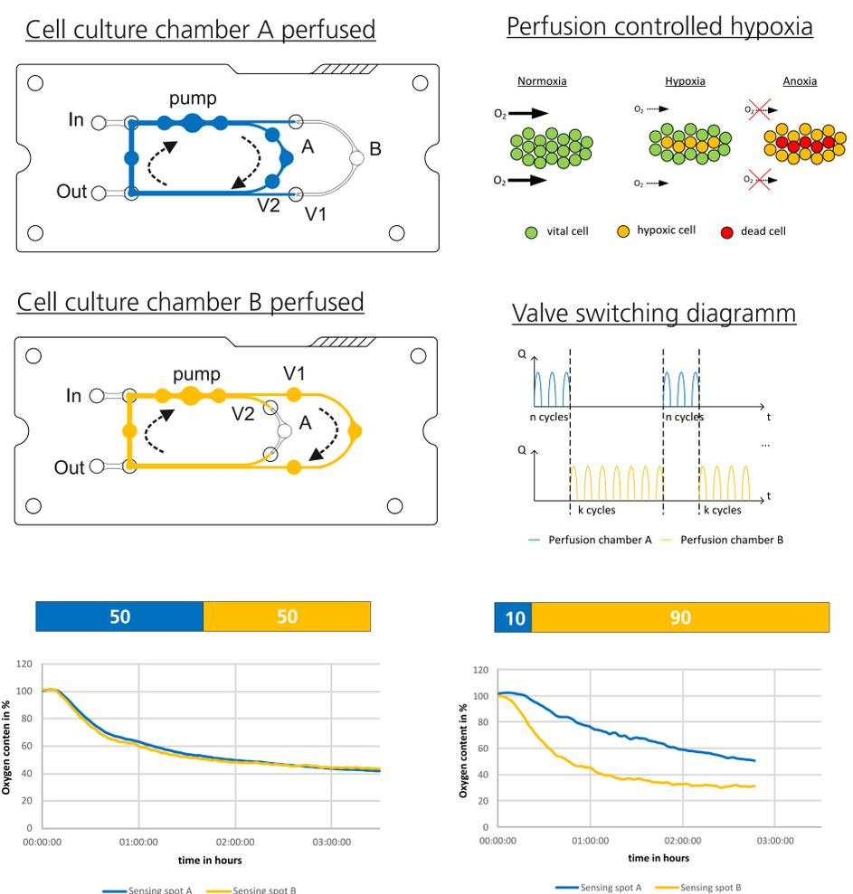
**FIGURE 2:** Top: Principle of perfusion controlled hypoxia assay with two parallel cell culture chambers A and B controlled by the closing valves V1 and V2. Bottom: Measured oxygen content in both chambers for different actuation cycles of V1 and V2 (50/50 and 10/90) under deoxygenation with nitrogen as process gas mimicking two different hypoxic states.
