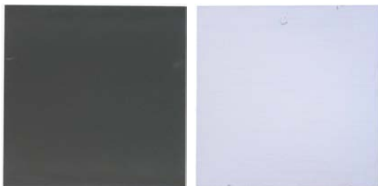
Fig. 6: Photos of the front (left) and the rear sides (right) of a 6 inch CZ Si wafer after alkaline texturing. The rear side was protected by an APCVD SiO 2 layer, which was subsequently etched in HF.
