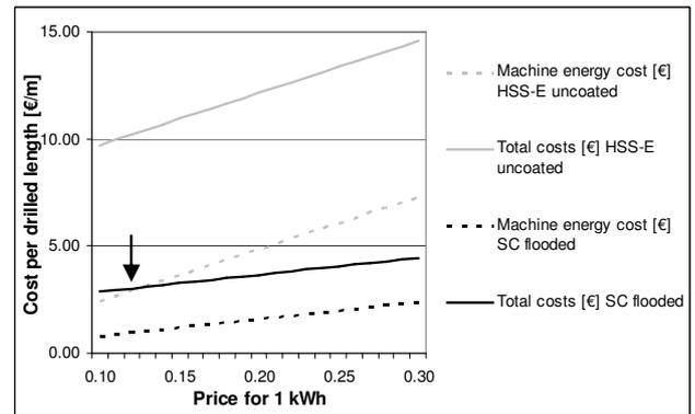
Figure 11: Influence of the price of one kilowatt-hour on the machine energy cost and total cost (Uncoated HSS-E and SC flooded)
