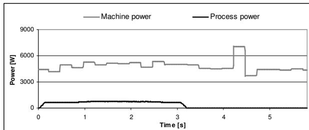
Figure 3: Machine power and process power during drilling with coated HSS-E drill
