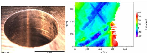
Figure 7: Burr shape of drilling EN-GJL-250 (SC flood cooling)
