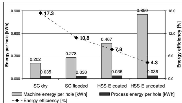
Figure 8: Process and machine energies per hole and machining efficiency factor for different drilling tools and cutting regimes
