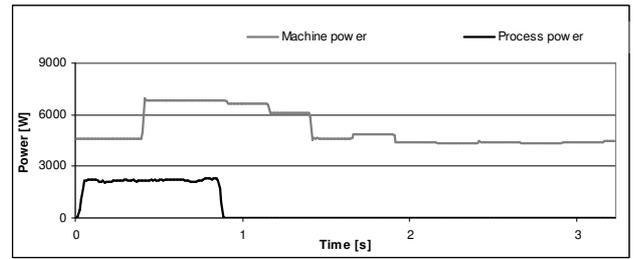
Figure 4: Active power and process power during drilling with coated SC drill (flood cooling)
