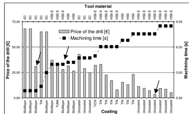
Figure 1: Drilling tool spectrum for machining a Ø7 x 35 mm bore on EN-GJL-250 cast iron
