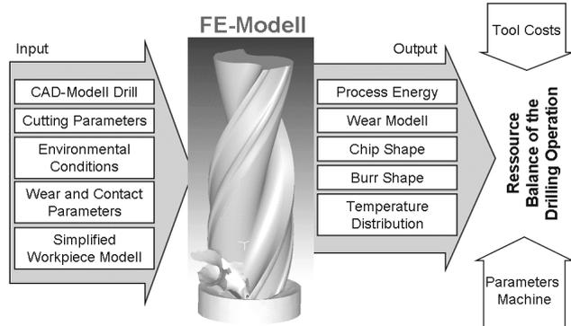
Figure 12: Numerical simulation for the determination of a resource balance
