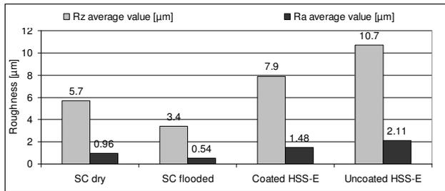
Figure 6: Surface roughness of the inner wall of the drilled holes
