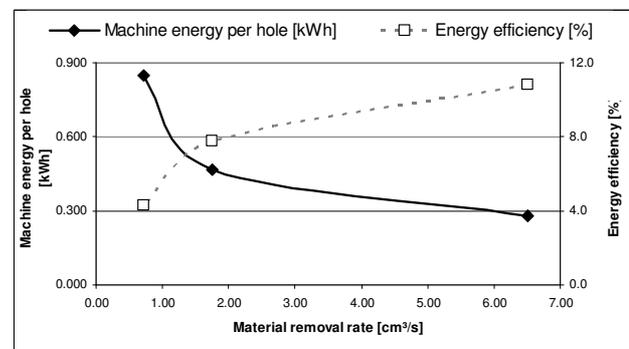
Figure 9: Influence of material removal rate on machine energy and energy efficiency
