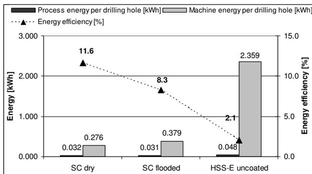
Figure 13: Numerically determined energy balance for drilling AISI-4140
