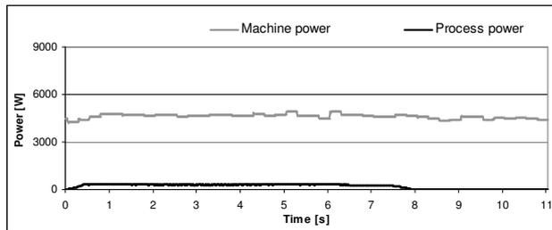
Figure 2: Machine power and process power during drilling with uncoated HSS-E drill
