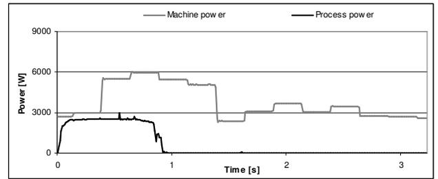
Figure 5: Machine power and process power during drilling with coated SC drill (dry)
