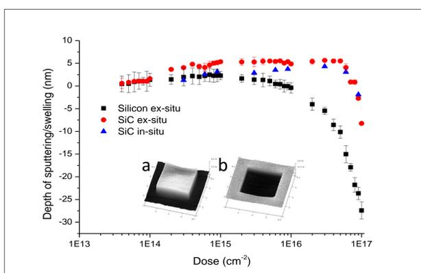
**Depth (or height) of irradiated structure (relative to non-irradiated surrounding) as a function of ion dose measured in Si (ex-situ) and SiC (ex-situ and in-situ). Inset: (a)Swelling and (b)sputtering in SiC**
