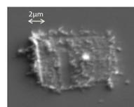
**Scratched bump (swollen region by Ga irradiation) in Si due to mechanical damage by AFM tip**
