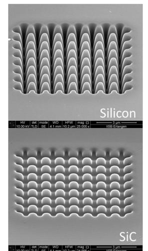
**Structures fabricated by milling horizontal & vertical lines\*\***
