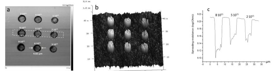
**(a) SSRM map of circles (diameter 4  $\mu$ m) irradiated with Ga ion dose ranging from  $1 \cdot 10^{15}$  to  $9 \cdot 10^{15}$  cm<sup>-2</sup>, (b) corresponding topography measurement in SiC and (c) sectional view of resistance in log(ohm).**
