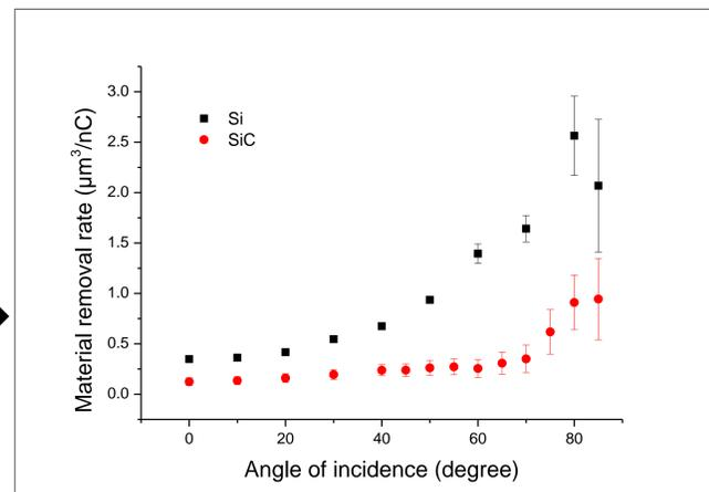
**Experimental angle dependent material removal rate for silicon\* and SiC for 30 keV Ga ion.**
