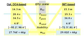
Figure 6: Comparison of the two floater designs for the DTU 10 *MW*
