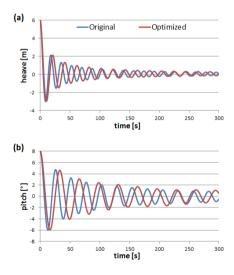
Figure 3: Motions of the optimized (solid) and original (dashed) OC4 semi-submersible platform designs (a) mean; (b) standard deviation
