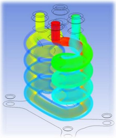
CFD simulation of channels
