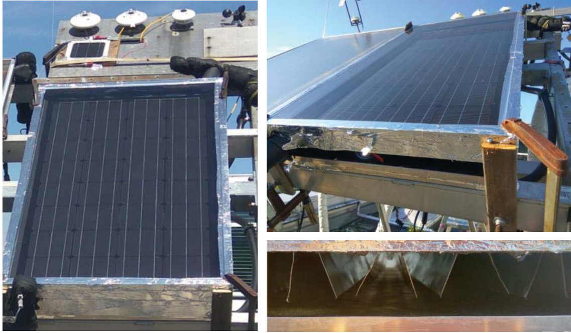
Figure 5.5: Photos of the PVT collector “PVT03-vented” during outdoor testing with closed vents (left) and opened vents (right).
