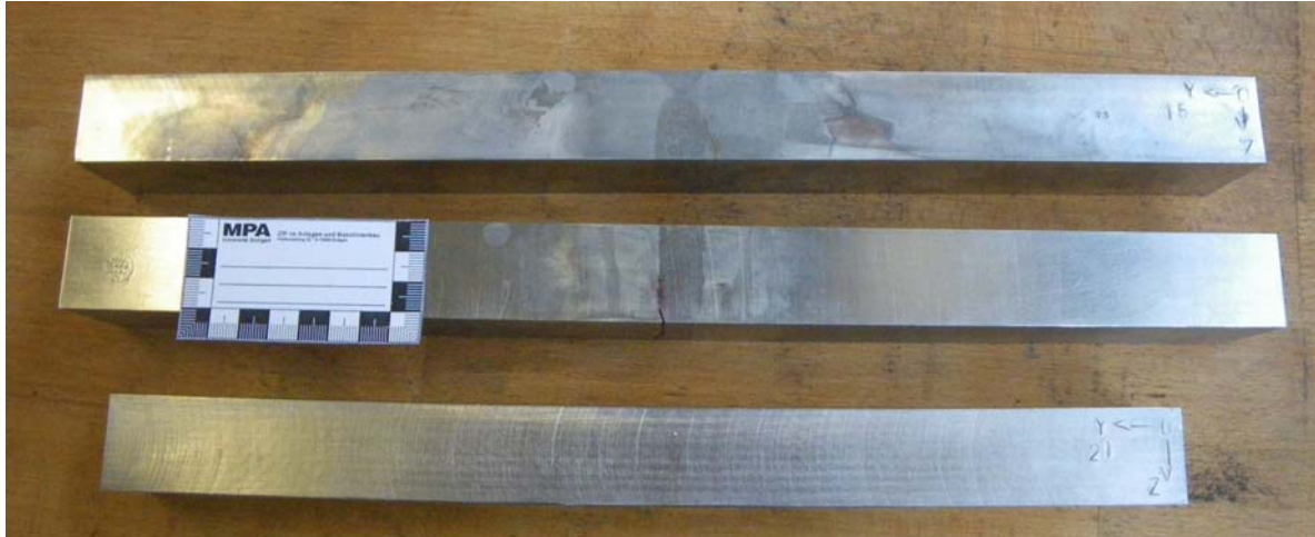
Figure 1. Austenitic test specimens with and without weld.
