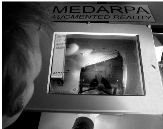
Fig. 3. AR window, the user navigates inside an anthropomorphic phantom to the red target region. The instrument has a green overlay.
