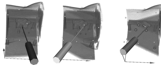
Fig. 4. The virtual overlay of the instrument changes colours: red for non-correct direction to target region, yellow for correct direction to target region and green, if the instrument's tip hits the target region.
