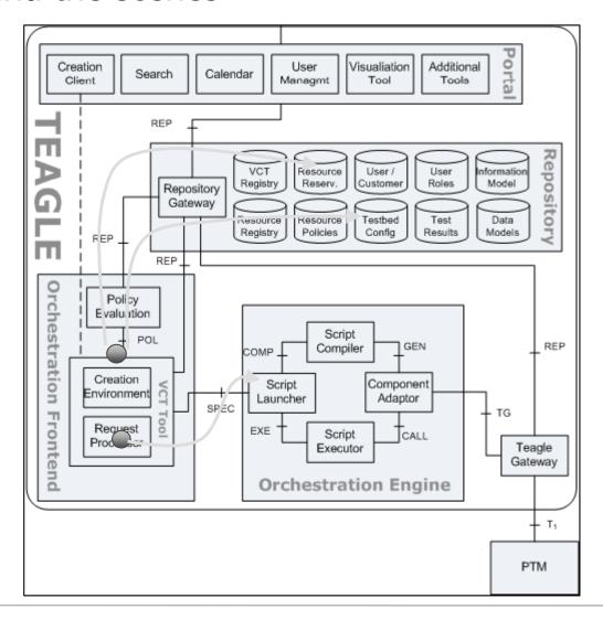
The Teagle tool helps reconfiguring the testbed and deploying new resource instances.
