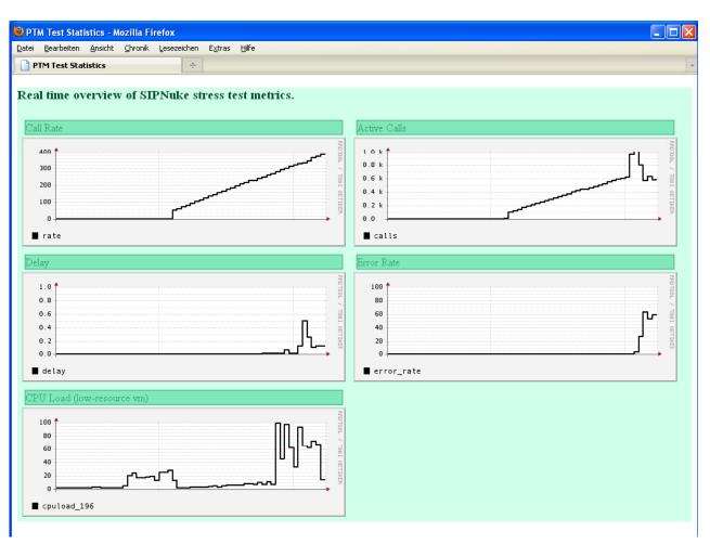
Execution of the first experiment. The CPU load of the small XEN reaches 100%, additionally the machine runs out of memory.
