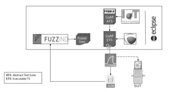
Figure I - Schematic overview of generating fuzzed data from already existing conformance tests.
