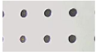
Fig. 3. Some detected local minima displayed as yellow crosses – hole-objects can be determined with sub-pixel accuracy
