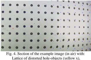
Lattice of distorted hole-objects (yellow x), corresponding lattice of undistorted locations (blue x), and image center (red +)
