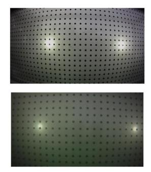
Fig. 2. Example pictures taken by pasUWP – above in air; lower in water
