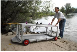
Fig. 1. Passive underwater inspection platform pasUWP of Fraunhofer-IOSB ready for launch on a slip ramp with calibration plate inserted
