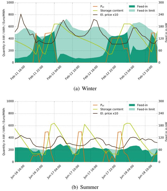
**Figure 5:** Exemplary sequence for operation of the P2G unit in the price use-case.
