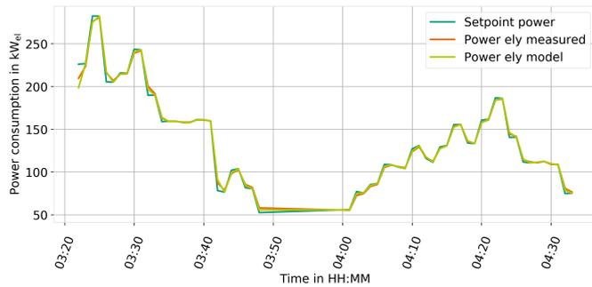
(c) Exemplary sequence to show the dynamic behaviour of modelled and simulated electrolysis mode.
