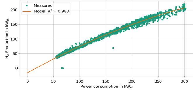
(a) Modelled and measured relationship between electrical power and hydrogen production.
