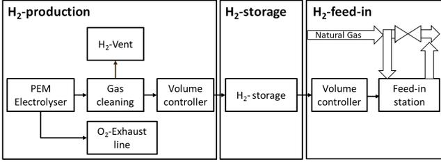
**Figure 2:** System description of the P2G test site at Fraunhofer ISE in Freiburg.
