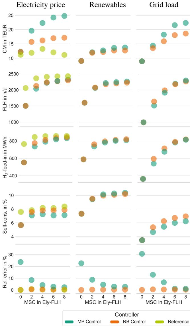
**Figure 8:** Sensitivity analysis of controls (coloured dots), storage size (x-axis) and use-case (columns) for different KPIs (rows). Storage capacities (MSC) are represented in full load hours (FLH) of the electrolyser.
