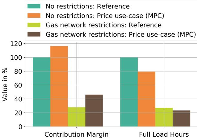
**Figure 7:** Influence of restrictions in the gas network on selected KPIs. Values are shown as relative numbers compared to the reference case without network restrictions. For simplicity Contribution Margin (CM) only considers electricity purchase and hydrogen sale.
