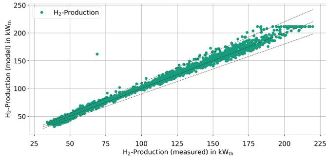
(b) Comparison of measured and simulated hydrogen production. Dashed lines represent the 10 % deviation corridor.
