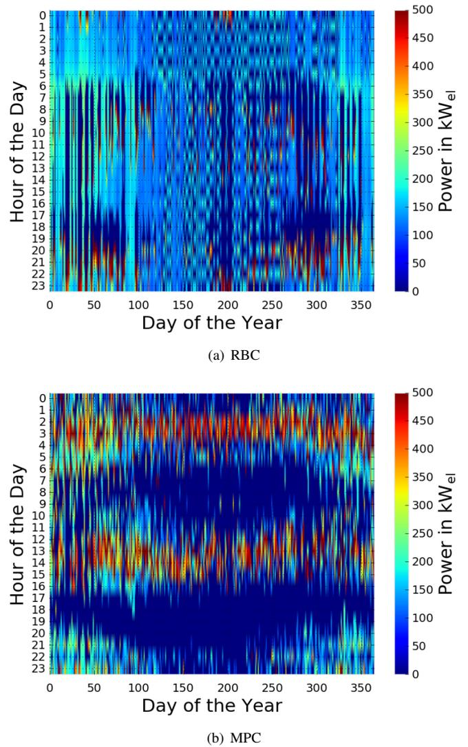
**Figure 6:** Operation of the electrolyser for every hour of the year in the price use-case for the rule-based controller (RBC) and the model predictive controller (MPC).
