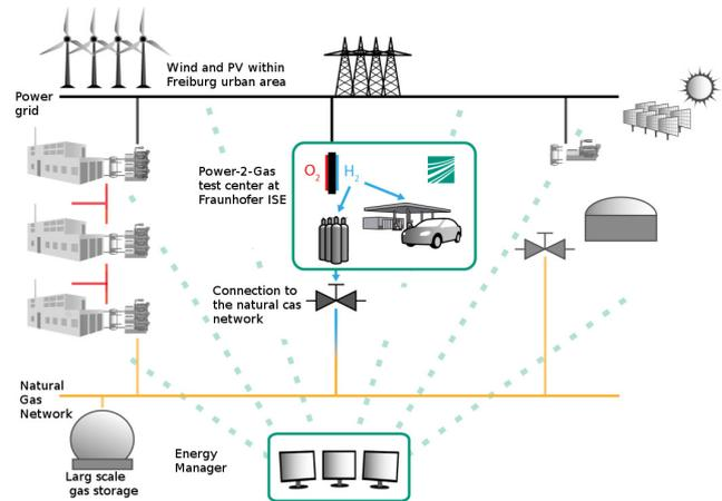
**Figure 1:** P2G stations as part of an urban energy system as will be demonstrated in the city of Freiburg, Germany.
