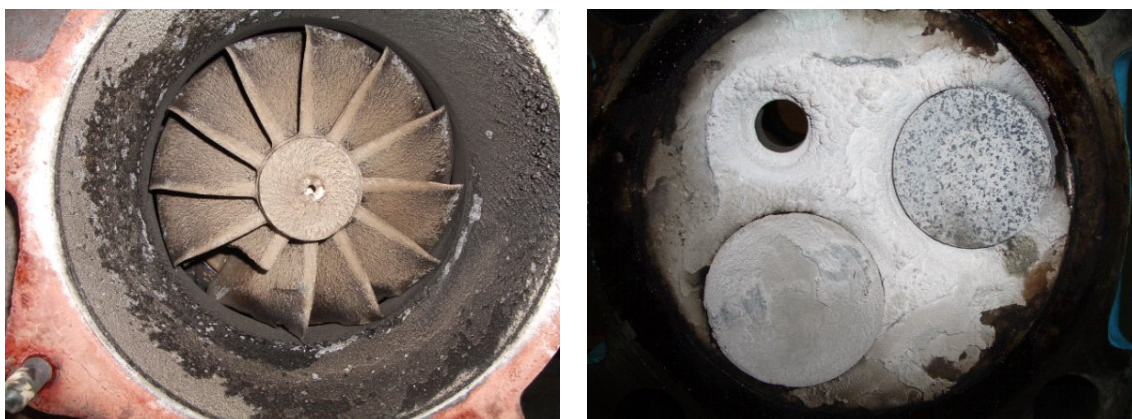
Fig. 1. Damaged blade wheel of a turbine caused by acid corrosion (left), \text{SiO}_2 -deposition on a cylinder head caused by siloxane decomposition (right), both after more than 3500 h of operation.
