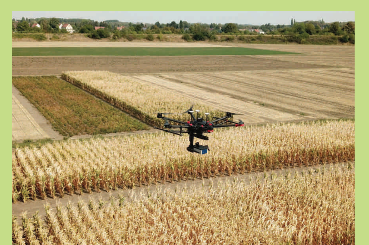
Additional multispectral drone trials (400-950 nm and thermal 7-13 \mu m) will take place in 2019.
