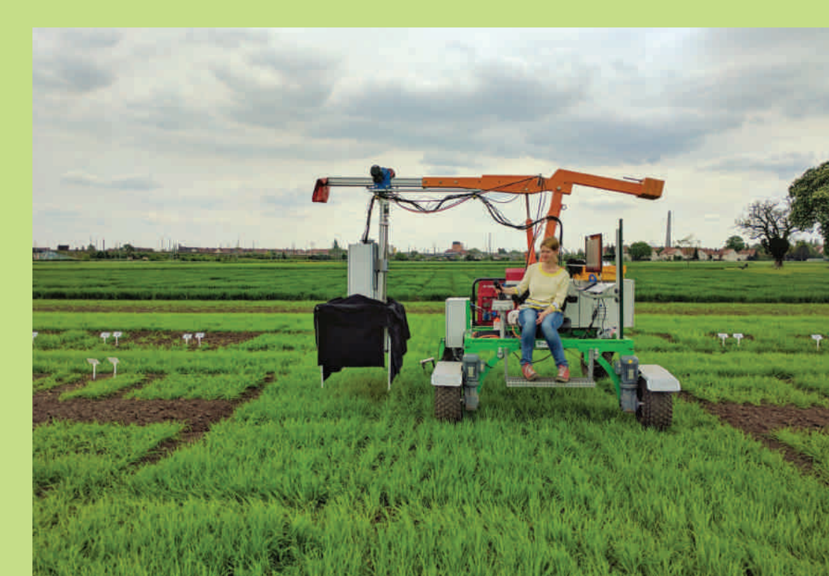
Hyperspectral imaging system "Agrover". The black sunlit-proof box contains both the hyperspectral- and the RGB-camera. QR code and GPS keep track of plant positions.
