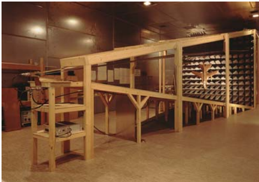
Fig. 1. TEM waveguide for EMC tests in Fraunhofer INT
