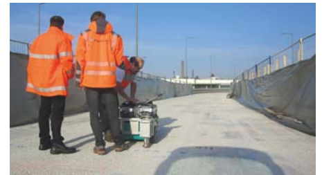
BetoScan for Bridge Deck Inspection
