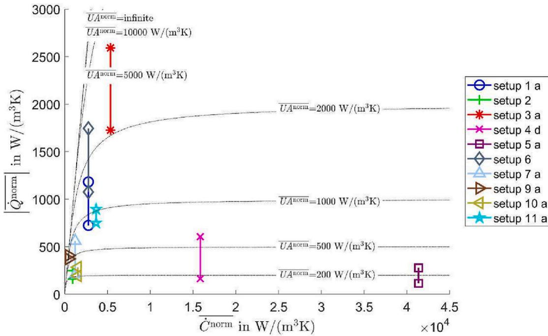
Fig. 9.  $\overline{Q}_{energy}^{norm}$  and  $\overline{Q}_{time}^{norm}$  with  $T_{ref} = T_{initial}$  plotted over  $\overline{C}_{energy}^{norm}$  for one experiment of every setup except for Setup 8 – for all cases  $\overline{Q}_{energy}^{norm} > \overline{Q}_{time}^{norm}$ .
