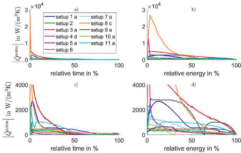
**Fig. 3.**  $\dot{Q}^{norm}$  with  $T_{ref} = T_{initial}$  plotted over relative time or over relative energy for one experiment of every setup. The plots c) and d) are zoomed in versions of the plots a) and b) respectively.
