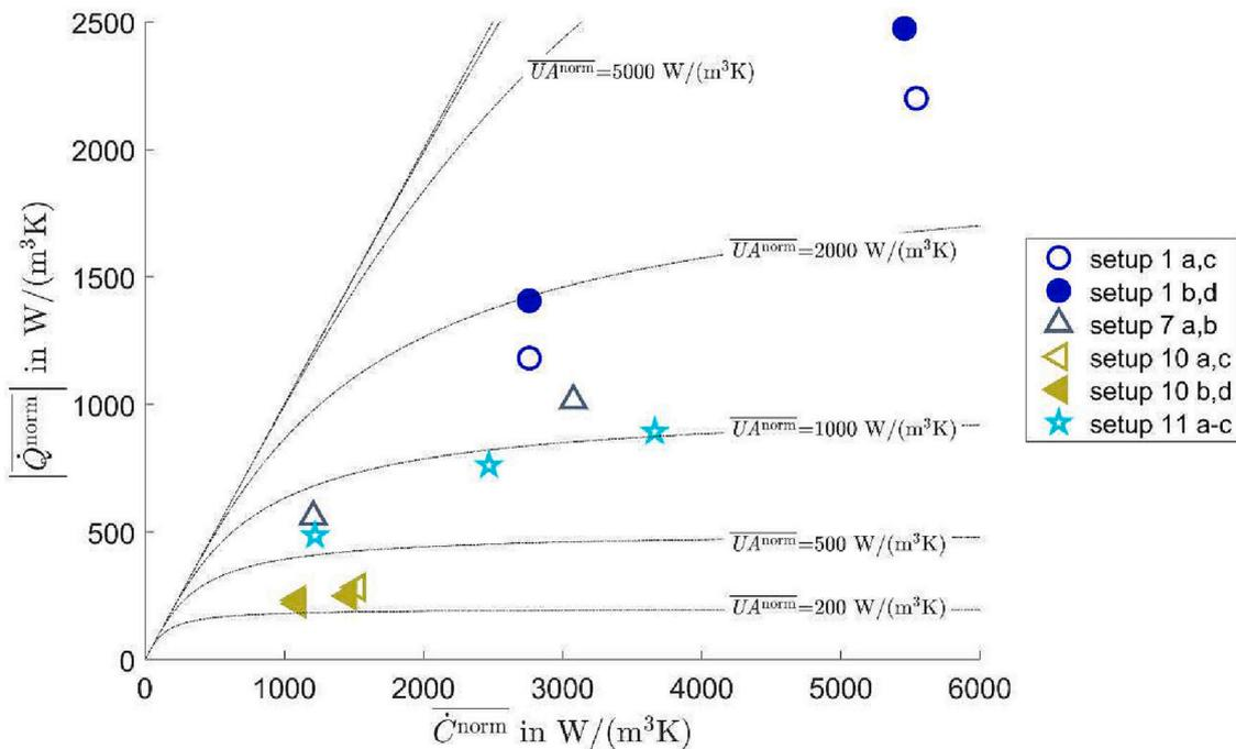
Fig. 11.  $\overline{Q}_{energy}^{norm}$  with  $T_{ref} = T_{initial}$  plotted over  $\overline{C}_{energy}^{norm}$  for experiments intended to be identical but with different mass flow.
