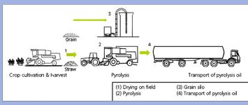
Fig. 3: logistic chain for mobile pyrolysis
