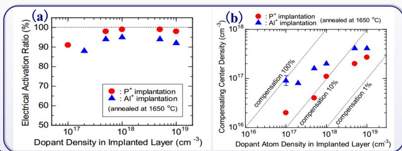
Fig 5. Changes in electrical activation rate and deep level defects with different ion implanted doses [1].
