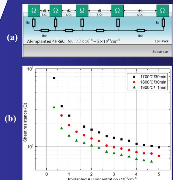
Fig 1. Sheet resistance measurement of Al implanted p-type 4H-SiC. (a) Schematic diagram of Transfer Length Model (TLM) structure sample; (b) Sheet resistance changes with the concentration of Al ions implanted and the annealing conditions.
