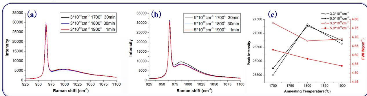
Fig 4. Raman results for Al-implanted 4H-SiC samples with different surface concentrations and annealing conditions.
