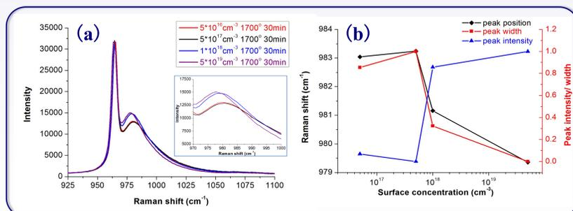
Fig 3. Raman results for Al-implanted 4H-SiC samples with different surface concentrations.
