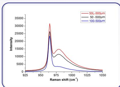
Fig 2. LO and LO+ Raman results for the same 4H-SiC sample using different objective lenses.
