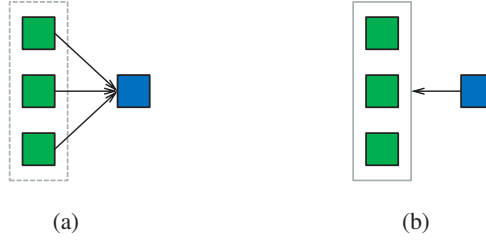
Figure 2.1: Green boxes represent database videos and the blue box represents a reference video. (a) Identification performs an identification task for each database sample video to the reference video. (b) Retrieval poses one search request to the database with the reference video as search pattern.
