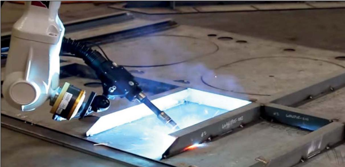
Figure 4: Computer Aided Robotic Welding (CAR-W) demonstrates value of connection to underlying product model at Bollinger Shipyards
