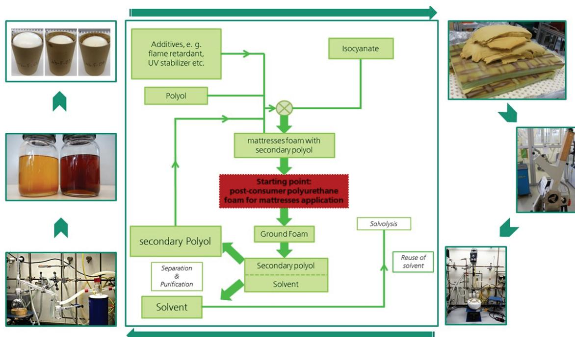
Figure 2: Chemical recycling scheme of glycolysis process
