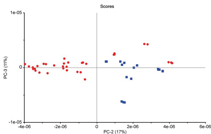
Figure 5: PC analysis applied for distinction of MDI (red)- and TDI (blue)-based polyurethane material
