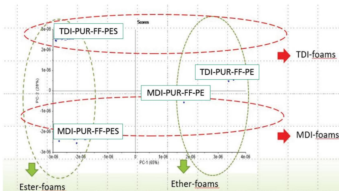
Figure 6: PC analysis for distinction of different polyurethane materials according to polyol and isocyanate component
