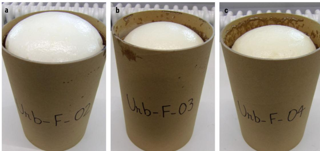
Figure 8: PU foams obtained using various ratios of secondary polyol (a) 10 phpp, (b) 20 phpp and (c) 30 phpp
