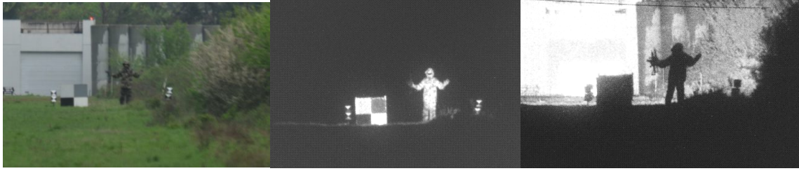
Figure 22. A soldier in uniform with a weapon in his left hand, range 800m. Left: visual, middle: 1550 nm active image in reflective mode, right 1550 nm active image in silhouette mode. The silhouette mode shows a double exposure. (Date 2013-04-11, time 18:26:05)
