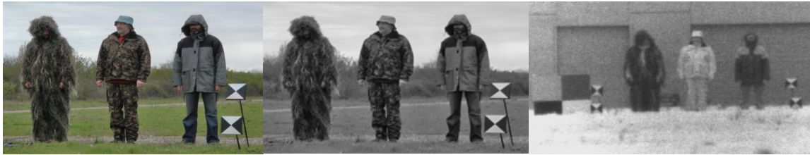
Figure 13. Clothes measured from 800m distance. Left: visual, middle:gray scale VIS image, right:passive NIR image. Clothes in each image, from left to right: Ghillie (Item J), 2: Swedish hunting (Item A) and blue cap, 3:Grey jacket (Onera) and jeans. (Scenario 50 2013-04-09 16:14)
