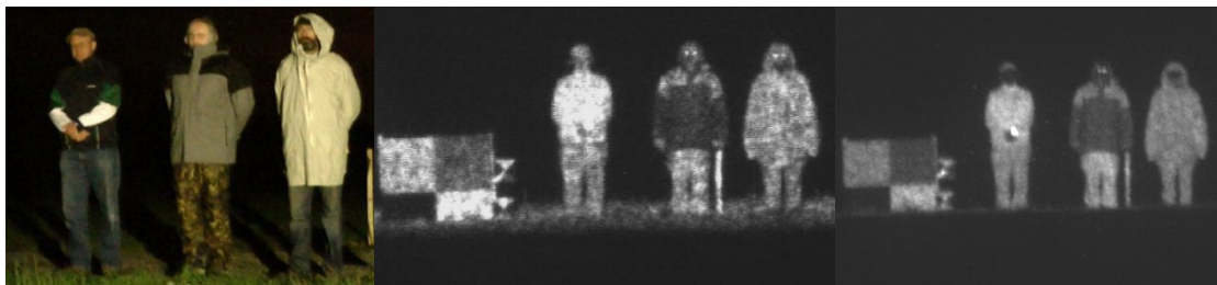
Figure 16. Clothes measured from 800m distance. Left: visual, middle: active NIR image, right: active 1.5 \mu\text{m} . Clothes from left to right in each image: Jogging dress, jeans and beige cap. 2: Grey jacket and Swedish hunting pants (A). 3: White anorak (item G), jeans (item H) and black cap. (Scenario 63, 2013-04-09 22:26:55)
