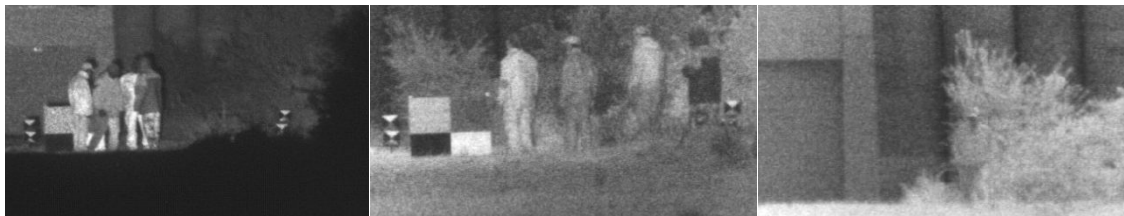
Figure 20. Clothes compared to background, range 1000m. Left: an active 1.5 \mu\text{m} image of a crowd against bushes and a concrete wall, middle: persons against the terrain for active 808 nm imaging, right: a person against the terrain at 808 nm. In the latter case the person is well camouflaged against the background. (2013-04-11, time 19:06:39, time 18:51:30, time 17:59:50)
