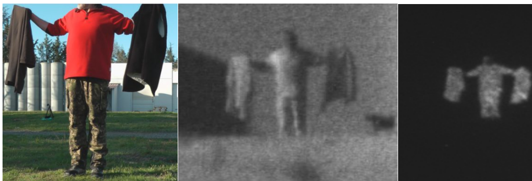
Figure 18. Clothes measured from 1000m distance. Left: visual, middle: passive NIR, right: active 1.5 \mu\text{m} . Clothes from left to right in each image: Black cotton to the left, red sweater (polyester) in the middle and white (and black) polyester to the right. (Scenario 54, 2013-04-10 18:54:05)
