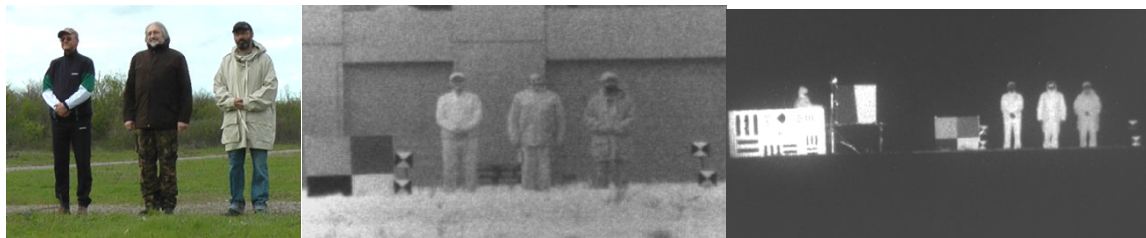
Figure 14. Clothes measured from 800m distance. Left: visual, middle: passive NIR, right:active 1.5 \mu\text{m} . Clothes from left to right in each image: jogging dress, Swedish hunting pants (Item A) and brown jacket, white anorak (Item G) and jeans (Item H). (Scenario 51 2013-04-09 18:03:15)
