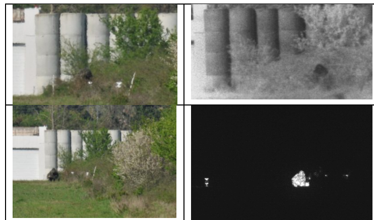
Figure 21. Person in a dark green uniform against bushes and a concrete wall, range 800m. Top left: visual, top right: passive 808 nm image. Bottom left: visual, right: 1550 nm active imaging using a 30 meter gate. (Date 2013-04-11 17:09:07 and 17:15:09)
