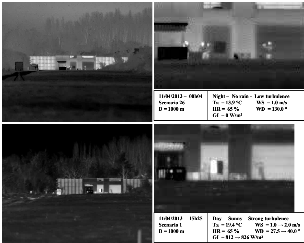
Figure 11. LWIR cooled sensor examples results for two scenarios: night – low turbulence (top) and day – sunny – strong turbulence (bottom).
