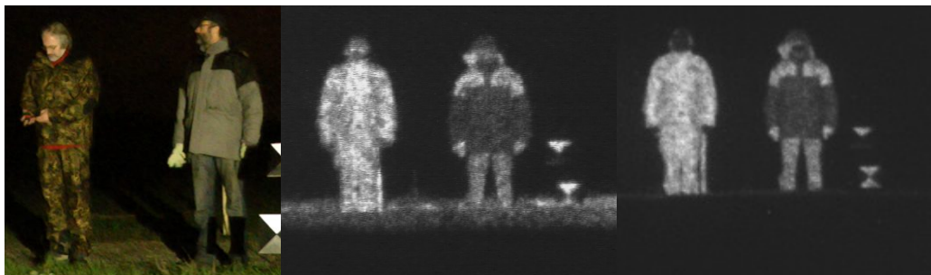
Figure 17. Clothes measured from 800m distance. Left: visual, middle: active NIR image, right: active 1.5 \mu\text{m} . Clothes from left to right in each image: 1: Uniform item F, jeans and beige cap, 2: Swedish hunting clothes and 3: grey jacket, jeans and black cap. (Scenario 60, 2013-04-09 22:10:55)
