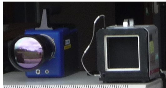
Figure 10. LWIR cooled sensor characteristics (left) and LWIR camera block along with the blackbody used for non-uniformity corrections (right)
