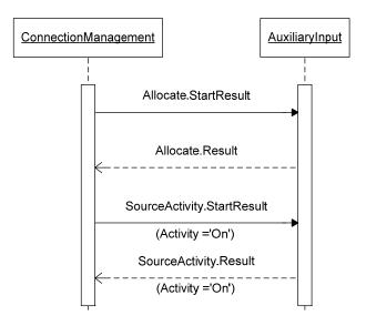
Figure 1 Example of a specified sequence for a successful startup of an Auxiliary Input [6]
