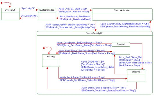
Figure 2 Example of the specification model for the Auxiliary Input Function Block [5]
