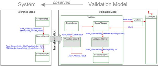
Figure 3 Validation model of the AuxiliaryInput Function Block [5]
