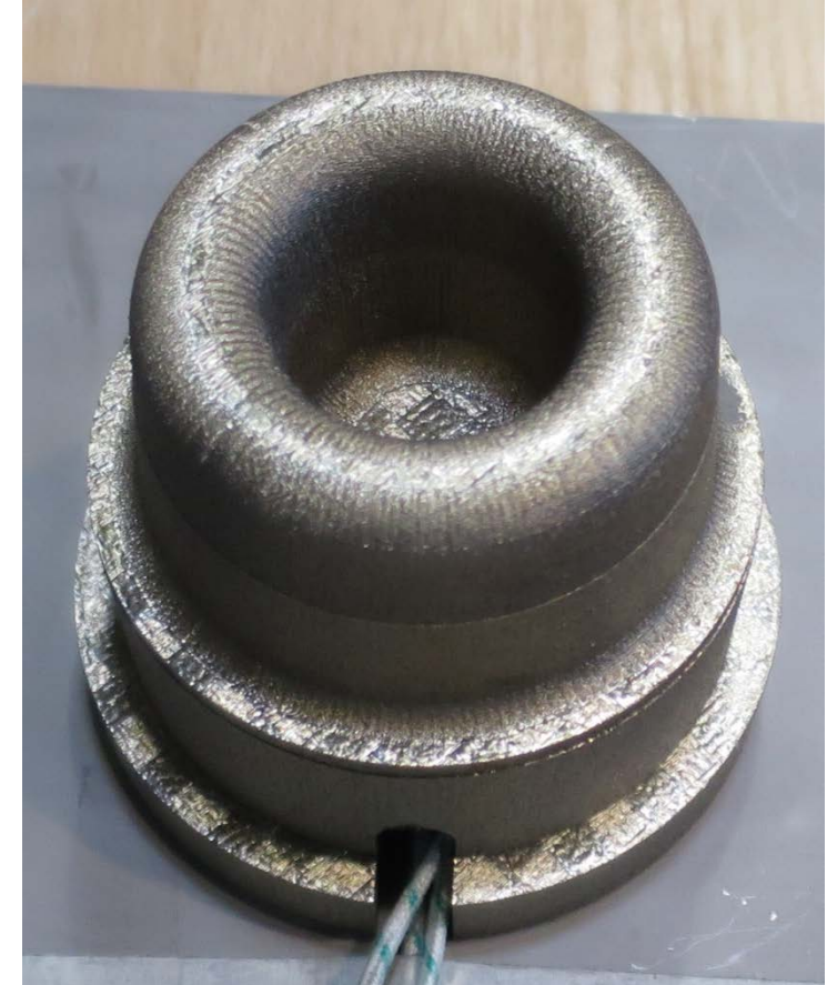
Additiv manufactured Uddeholm AM insert with 3 thermocouples
