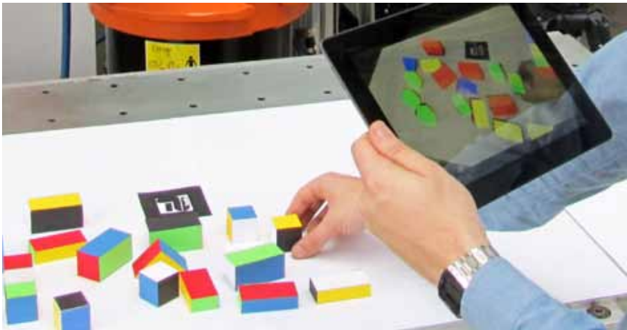
Easy programming: the human operator shows how it is done and the Tablet PC follows suite
