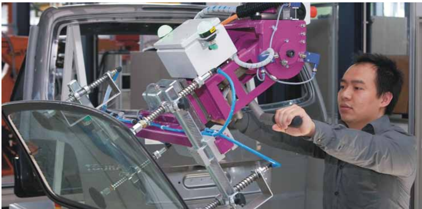
Semi-automatic windscreen assembly by cooperative robots
