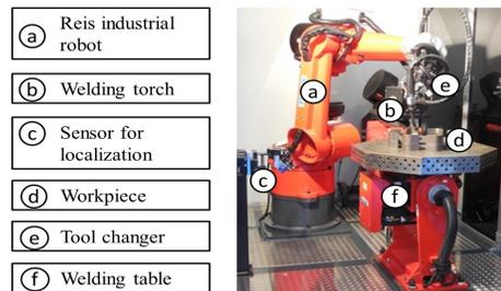
Fig. 4. Welding robot cell
