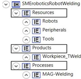
Fig. 5. Robot system semantic description in AML using the PPR model
