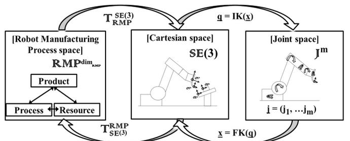
Fig. 2. Spaces for the optimal motion generation in robotic manufacturing
