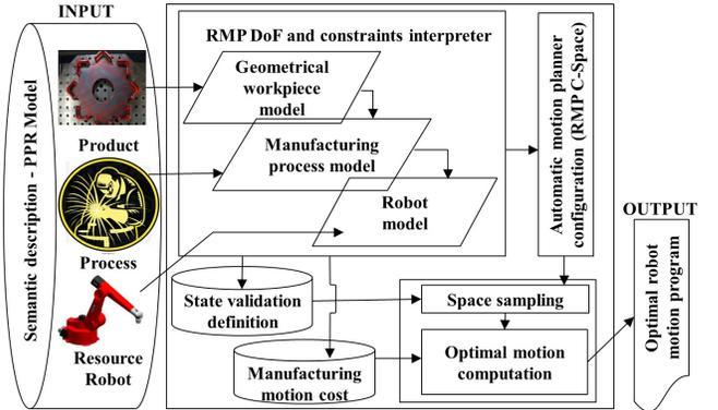
Fig. 1. Architecture for the automatic offline optimal motion generation for robotic manufacturing processes (DoF: Degree of Freedom)
