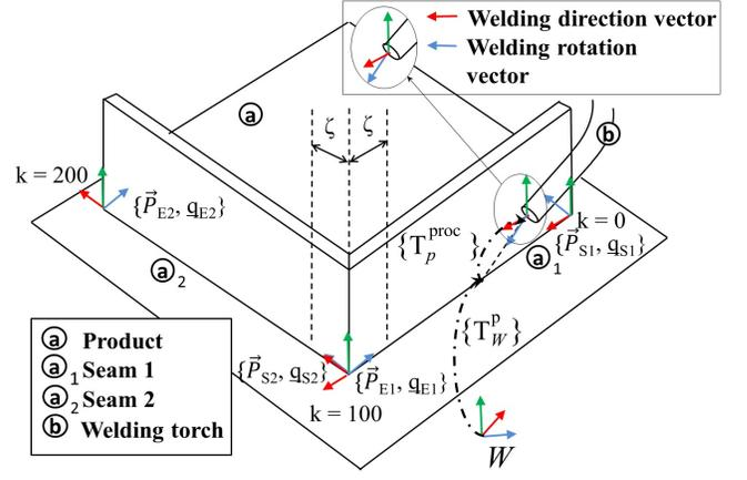
Fig. 3. Illustration of the T-Weld seam product model components and notations
