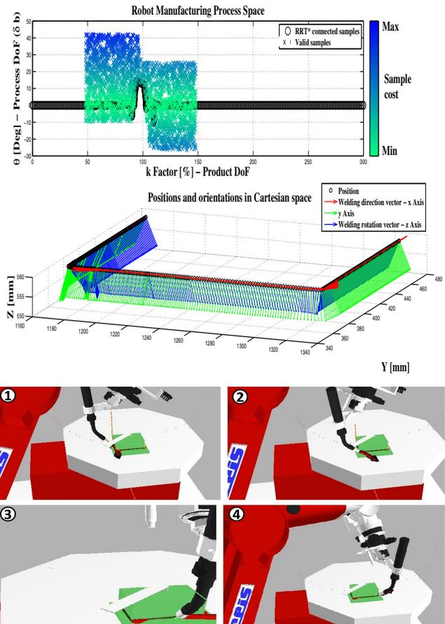
Fig. 8. (Up) Evaluated valid samples and optimal interconnected solution in the Robot Manufacturing Process space for avoiding a collision using the rotation around the welding direction vector for multiple seams (Middle) Cartesian space with the plot of the found optimal welding direction vector (Down) Sequences of Robot movements in the simulated robot scene for the optimal collision avoidance
