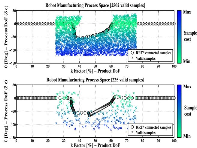
Fig. 7. Evaluated valid samples and optimal interconnected solution in the Robot Manufacturing Process space for avoiding a collision using the rotation around the welding rotation vector for (Up) 2502 and (Down) 225 valid samples
