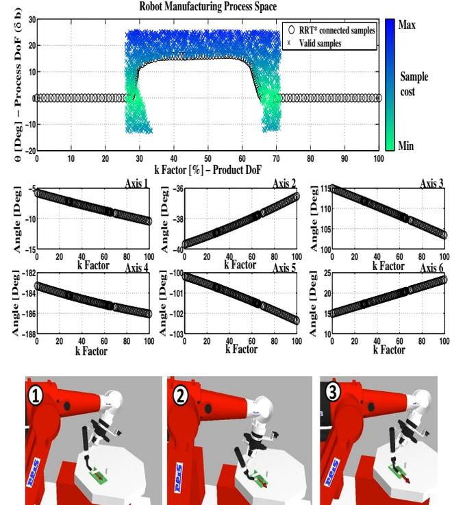
Fig. 6. (Up) Evaluated valid samples and optimal interconnected solution in the Robot Manufacturing Process space for avoiding a collision using the rotation around the welding direction vector (Middle) Joint space with the found optimal solution (Down) Sequences of robot movements in the simulated robot scene demonstrating the optimal collision avoidance
