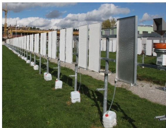
Figure 1. Vertical test panels used during leaching outdoor tests in Valley, Germany.
