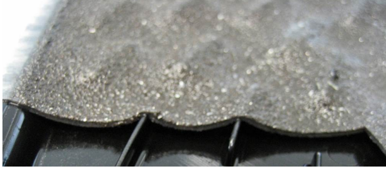
Figure 6.4: Bending of a filter under extreme loading conditions. The photo is courtesy of IBS Filtran
