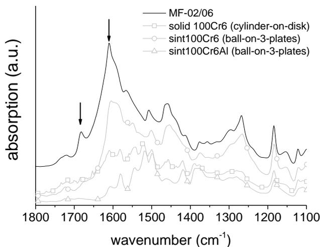
Figure 12: IR-spectroscopy of new and used MF-02/06 after friction test with solid 100Cr6 (cylinder-on-disk test, Figure 5), Sint100Cr6 and Sint100Cr6Al (ball-on-3-plates test, Figure 9)
