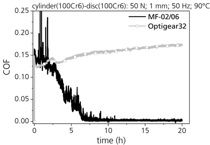
Figure 5: Reciprocating cylinder-on-disk friction tests using MF-02/06 and Optigear 32 as lubricant (100Cr6; 50 N; 1 mm; 50 Hz; 90 °C) [11]
