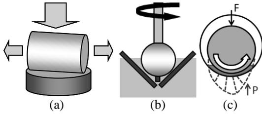
Figure 3: Geometry of model friction tests: (a) reciprocating cylinder-disk; (b) rotating ball-on-3-plates; (c) radial bearing
