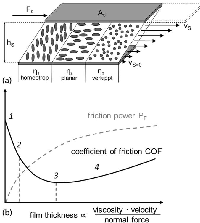
Figure 1: (a) Schematic illustration of the three Miesowicz viscosity coefficients of a liquid crystals aligned in a shear gap [20], [28], [29]; (b) Stribeck-curve with the different lubrication regimes: 1) boundary-, 2) mixed-, 3) thin-film- and 4) fluid-film-lubrication [44], [45]
