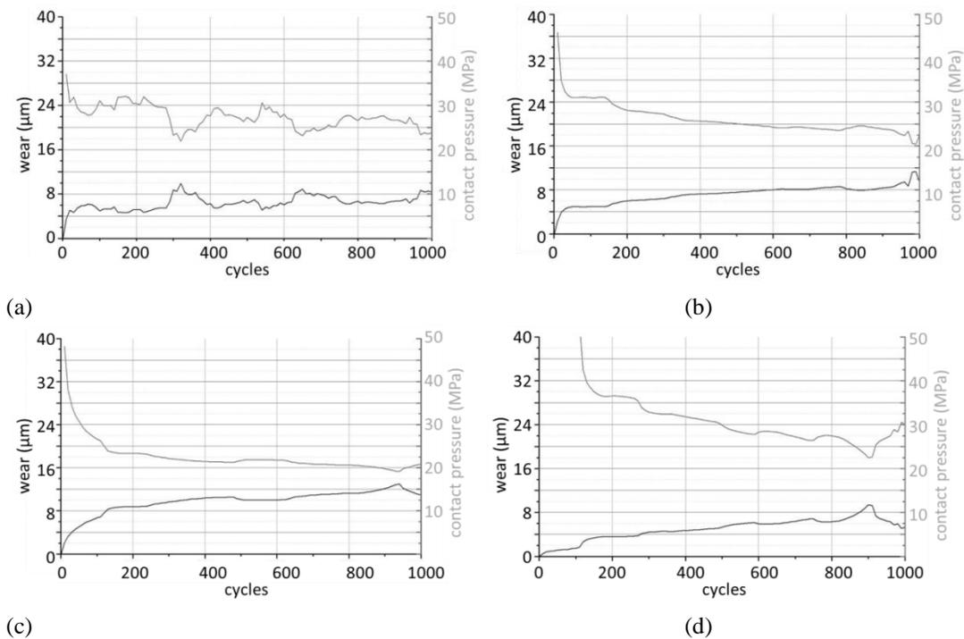
Figure 11: In-situ wear analysis using radial sintered iron bearings lubricated with the reference oil and the modified M1231 ( $\phi 2.5$  mm; 35 N; RT): a) Reference oil using sintered 100Cr6; b) Reference oil using sintered 100Cr6Al; c) M1231 using sintered 100Cr6; d) M1231 using sintered 100Cr6Al
