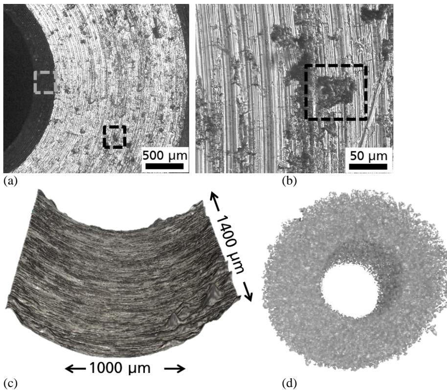
Figure 4: 100Cr6 sintered bearing before tribological testing (innerØ 2.5 mm): a), b) Analysis of frontal area using digital light-optical microscope (pore: 35 x 45 µm); c) Analysis of the friction surface of the bearing using laser scanning microscope; d) Analysis of the pore volume using computer tomography
