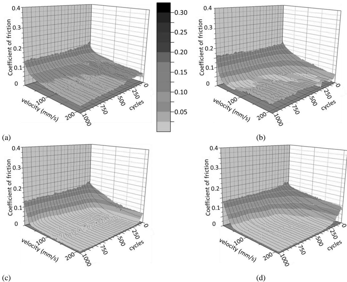
Figure 10: Friction tests using radial sintered iron bearings lubricated with the reference oil and the modified M1231 ( $\phi 2.5$  mm; 35 N; RT): a) Reference oil using sintered 100Cr6; b) Reference oil using sintered 100Cr6Al; c) M1231 using sintered 100Cr6; d) M1231 using sintered 100Cr6Al
