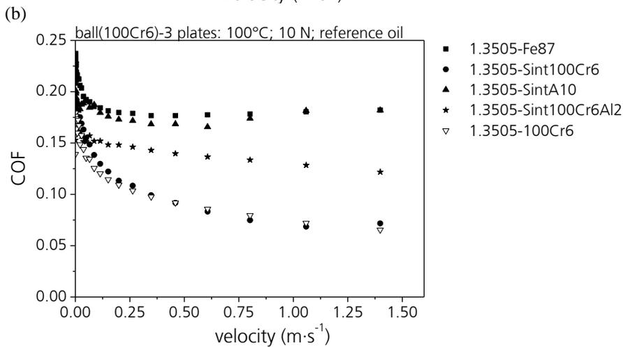
(c) Figure 7: Results of multi-tribotest with rotating ball-on-3-plates geometry using different sintered materials (100Cr6; 10 N; 100 °C): (a) Overview of the static friction values of MF-02/06 and reference oil using rotating ball-on-3-plates geometry; (b) Stribeck-curves (0-0.47 m/s) using MF-02/06; (c) Stribeck-curves (0-0.47 m/s) using reference oil
