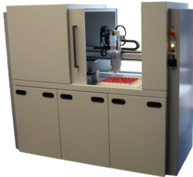
Figure 1: The automated CT scanner with sample changer
