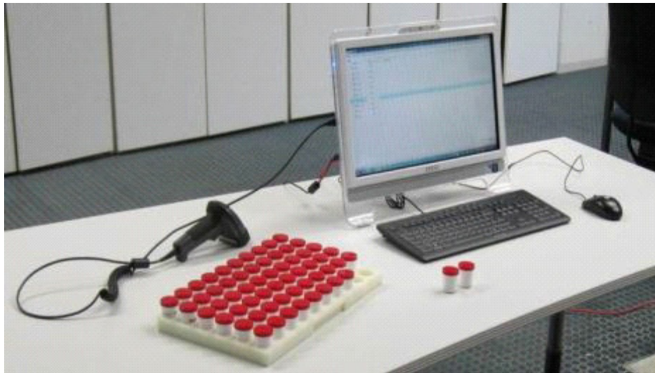
Fig. 1: The sample preparation station of the automated CT scanner
