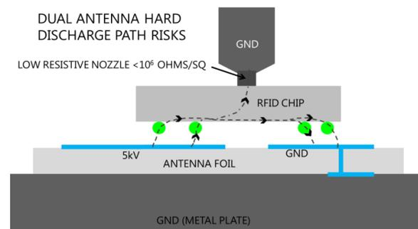
Figure 3: When a low-resistive rubber nozzle is used, a part of the voltage is discharged through the silicon substrate, where the ESD pad protective structures help bypassing sensitive circuitry. However, due to the low-resistive nozzle type, it is still a dangerous hard discharge scenario.
