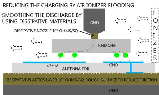
Figure 5: In addition to the scenario of Figure 4, the process chamber is flooded with ionized air, which makes the discharge very smooth and starts it already long before the device approaches to critical sparking distance to the antenna foil. Only very small charge remains in that case, being uncritical for the chip.
