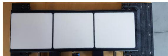
Figure 12: The improved indexer plate – frame out of dissipative material – gave already very good results in the trial runs – no main failing position (3 and 5 for 6x antenna matrix) any more.
