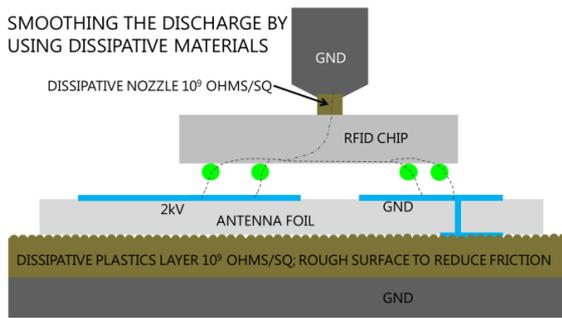
Figure 4: In this case, the nozzle is made from high-ohmic dissipative (about  $10^9$  Ohms/sq) rubber and the support includes a surface layer (>2 mm) of dissipative plastics. By this, the discharge is smoothed to very low current in order to avoid damaging the device.
