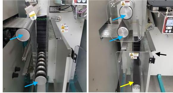
Figure 14: Blue arrows = old wheels, yellow arrow = new wheel construction with internal brushes to guarantee earth connection, black arrow = new soft dissipative brushes which can be used contactless as long as the distance to the surface to be discharged is  $< 3$  mm.
