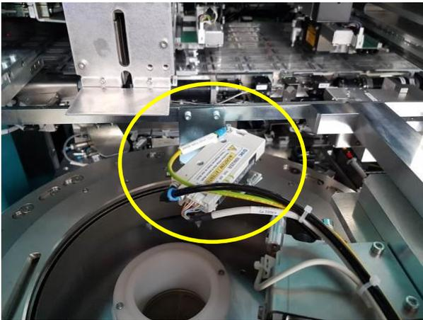
Figure 7: Die picking station, here with air ionizer.
