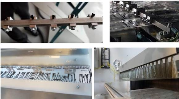
Figure 13: Soft dissipative brushes can be used both in a touching manner as well as non-touching corona dischargers. If the foil rollers are made from dissipative material, too, most air ionizers can be replaced by brush solutions.
