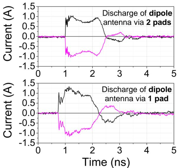
Figure 17: CDM stress of one coil antenna pad, discharging the capacitance of the dipole antenna via both pads (top) and via only one pad (bottom) through the chip under test condition TC 125 of ANSI/ESDA/ JEDEC JS-002-2014 [8]. The corresponding setups for the discharge via two or one antenna pad are illustrated in Figure 16 without or with the optional line cut.
