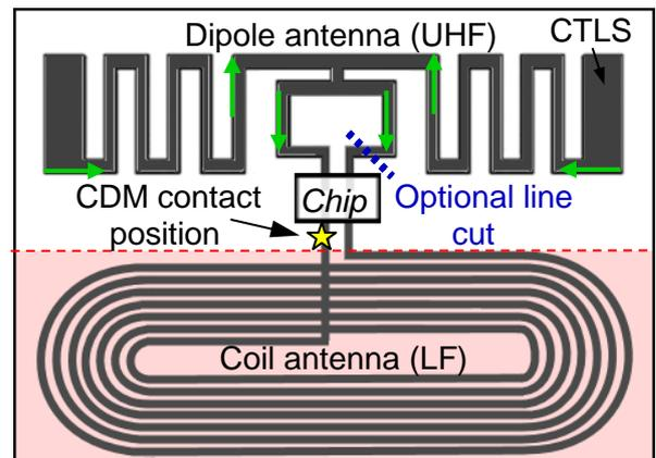
Figure 16: Exemplary schematic of a dual frequency RFID inlay with a multiple-folded open dipole (top) and a coil antenna (bottom). The discharge of the capacitance of the dipole antenna via two pads is measured by performing CDM on a coil antenna pad (★), while the rest of the coil antenna is cut (red area).
