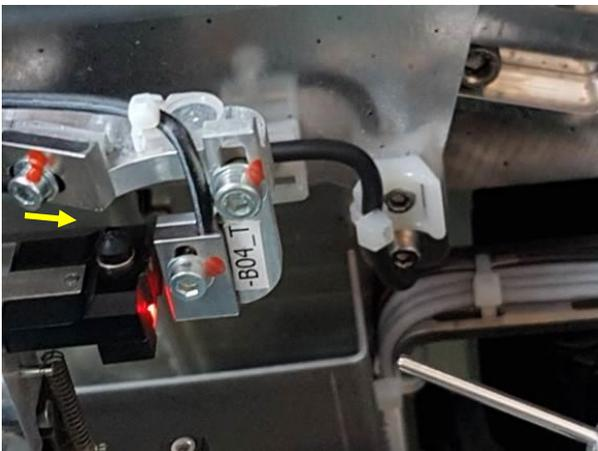
Figure 8: Picking nozzle to take the dies from the blue tape.
