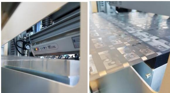
Figure 10: Inlay support conversion from metal (left) to a dissipative version (right).
