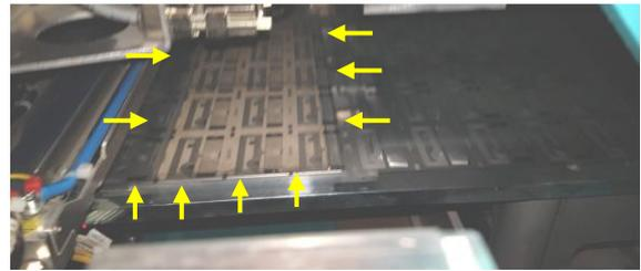
Figure 11: Vacuum tube support Al-blocks which can be proven to be the root cause for hard discharges and low yield at position 3 and 5 of a 6x inlay matrix. Covering them with paper tape/masking tape improves the yield on these positions, but a hard discharge path remains due to the Al-frame (yellow arrows) of the die placement vacuum support plate under the inlay.
