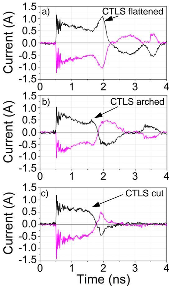
Figure 19: Current waveforms of the discharge of a half dipole antenna for different curvatures of the “Capacitive tip loading structure” (CTLs) (Figure 16) measured under test condition TC 125 of ANSI/ESDA/ JEDEC JS-002-2014 [8].
