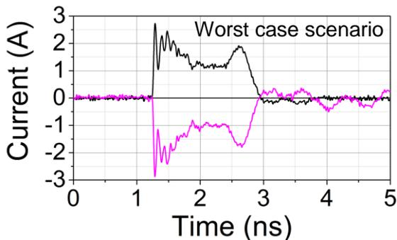
Figure 20: Worst-case scenario of the dipole antenna discharge via both pads through the chip by placing the foil on the insulating surface coating of the metal chuck. Apart from the lack of the dielectric FR4 plate, the test is performed under test condition TC 125 of ANSI/ESDA/ JEDEC JS-002-2014 [8].
