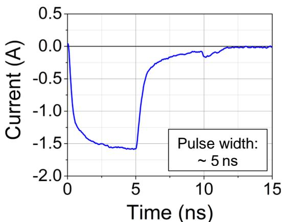
Figure 15: Current transient of VF-TLP on bare die.
