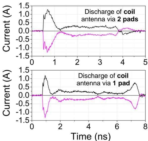
Figure 18: CDM stress of one dipole antenna pad, discharging the capacitance of the coil antenna via both pads (top) and only via one pad (bottom) through the chip under test condition TC 125 of ANSI/ESDA/ JEDEC JS-002-2014 [8].
