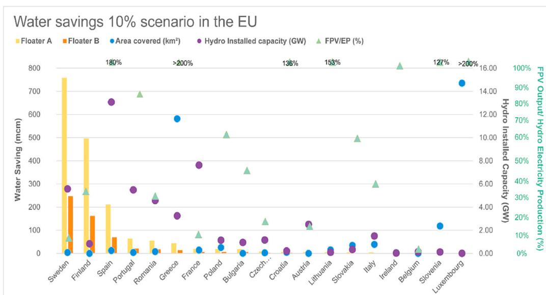
**Fig. 8.** Water saving after the installation either of floater A or floater B (suspended) in the EU for the 10% area scenario. The countries are sorted based on the water savings (larger to smaller).
