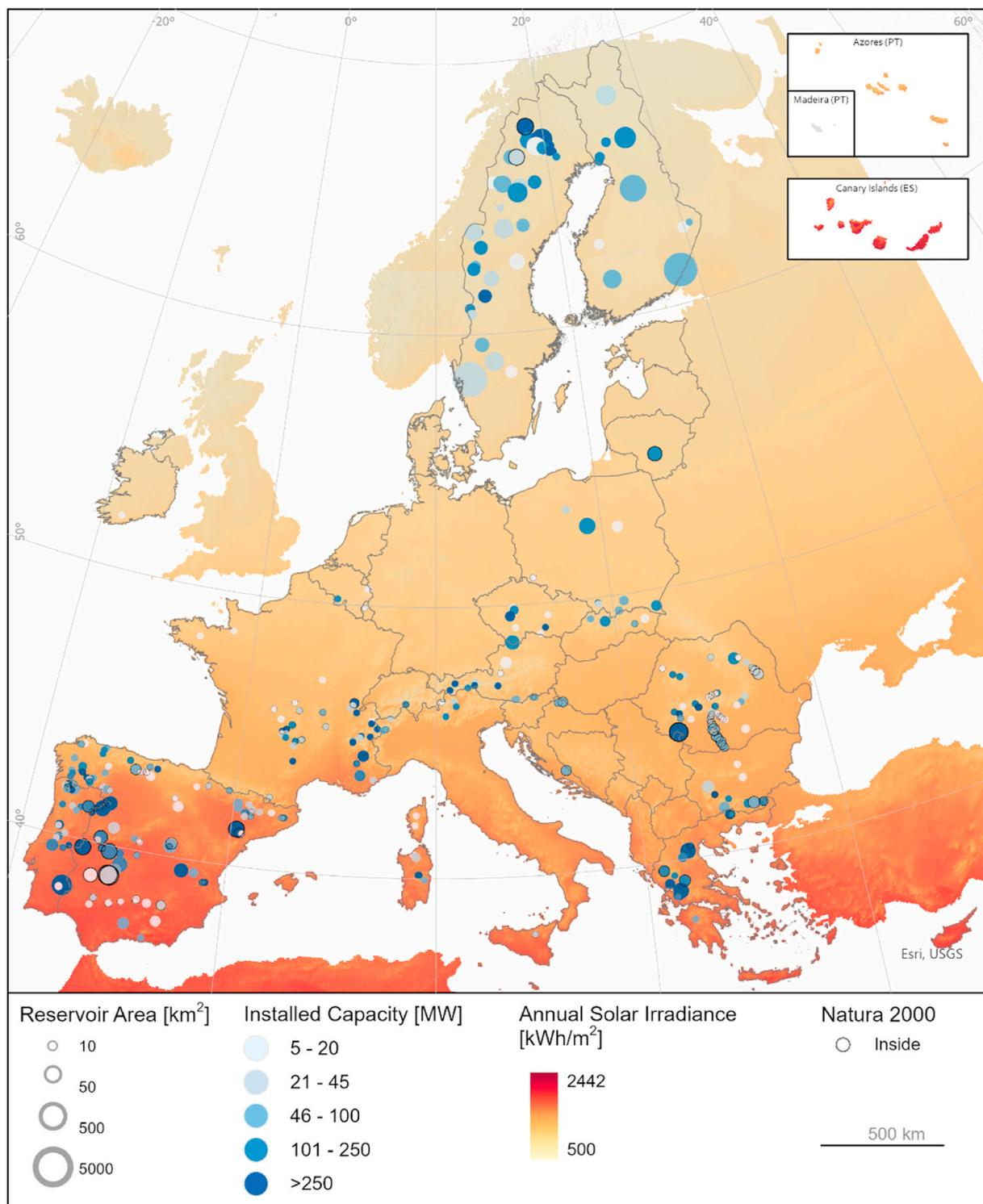
**Fig. 2.** Hydropower plants and corresponding reservoirs selected for the analysis are represented in circles. The assorted circles' colour indicates the installed hydropower capacity [MW] and the circles' size the corresponding reservoir area [km<sup>2</sup>]. Points with a black outline represent reservoirs inside the Natura 2000 sites. The background map represents the annual solar irradiation in [kWh/m<sup>2</sup>], (source PVGIS JRC).
