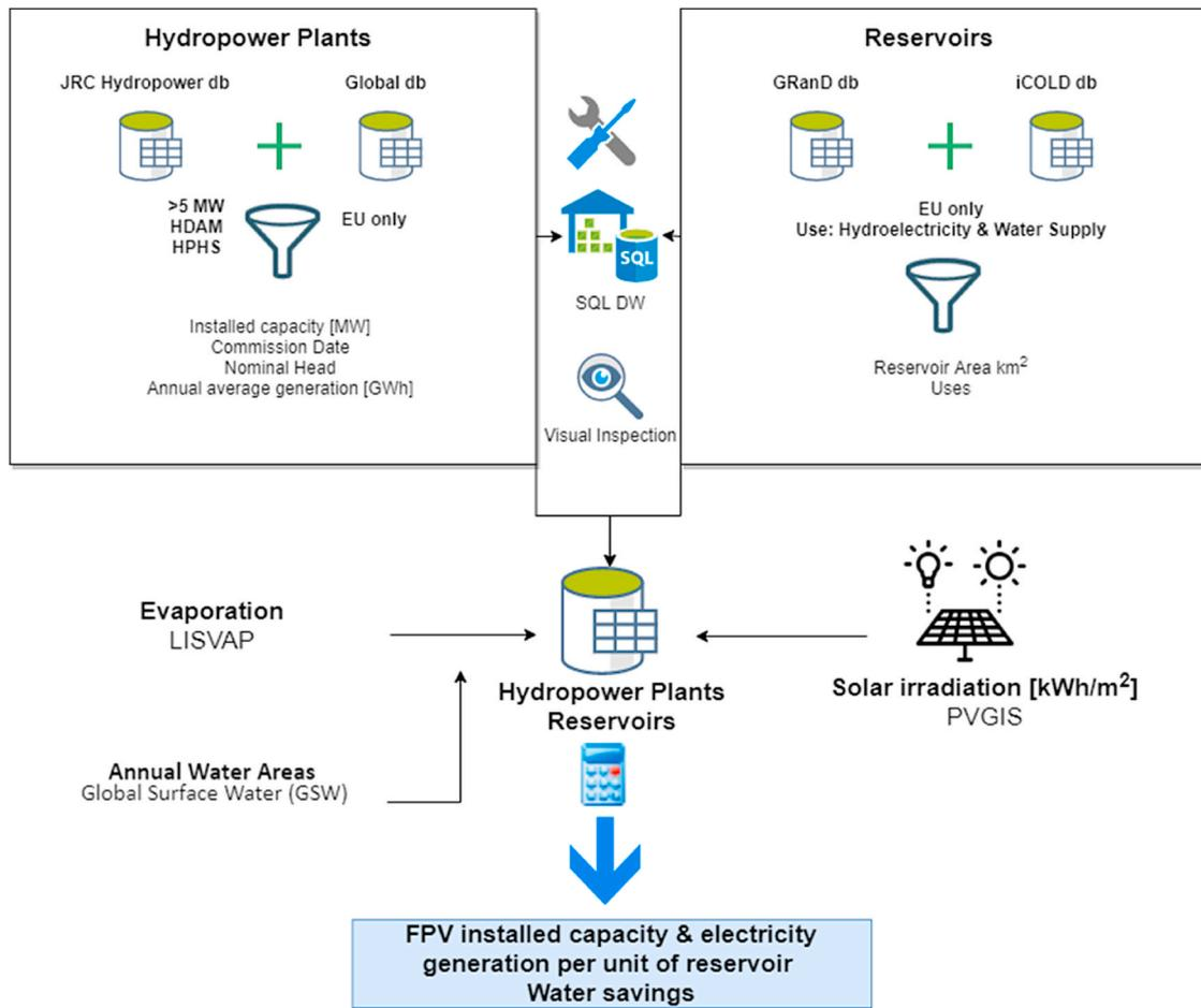
Fig. 1. Graphical representation of the methodology, databases and datasets used in the study and the final outputs.
