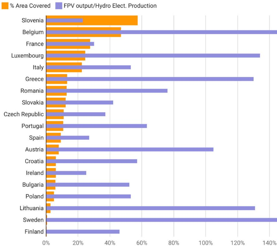
**Fig. 6.** Percentage of total area covered by FPV and the percentage of the total generated FPV output with the hydro electricity generation per EU27 country analysed for the HEIC scenario.
