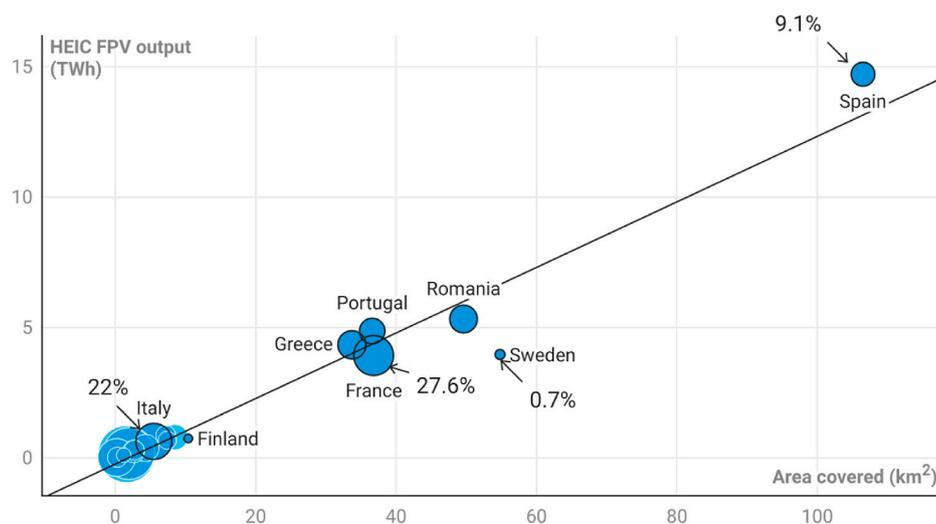
Fig. 5. Potential electricity output in TWh from installing FPV arrays for the HEIC scenario at EU level. The size of the circle indicates the percentage of area covered in HEIC scenario; some area covered percentages are indicated in labels.
