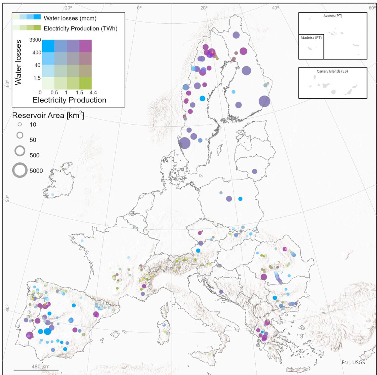
**Fig. 7.** Bivariate map for each reservoir in the analysed countries. The colours represent the water loss due to evaporation (mcm) and hydro electricity production (TWh). The circle's size indicates the reservoir's surface area in km<sup>2</sup>.
