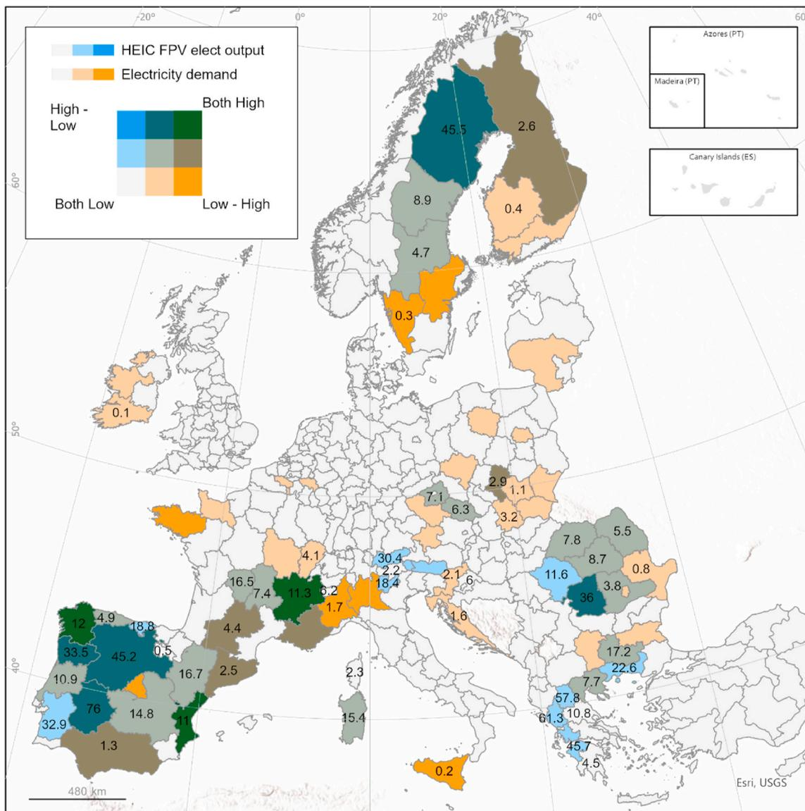
Fig. 9. Bivariate map with the FPV electricity output in the HEIC scenario and the electricity demand at NUTS2 level. The numbers represent the percentage between annual FPV potential generation with the HEIC scenario and regional total electricity demand.
