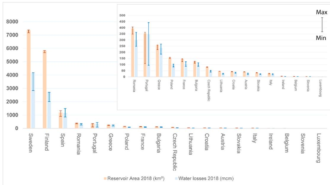
Fig. 3. Bar graph of the total reservoir areas and water losses of year 2018 and related minimum and maximum values for the period 2000–2018 aggregated at national level. Enlarged detailed view of the bar graphs for the countries with values of reservoir area and water losses less than 500 km<sup>2</sup> and mcm, respectively.
