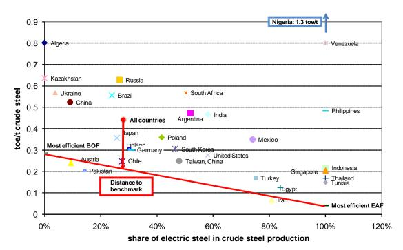
Figure 6: Unit consumption per ton of steel as a function of the share of electric arc furnace (EAF) steel in total crude steel production (2007)
