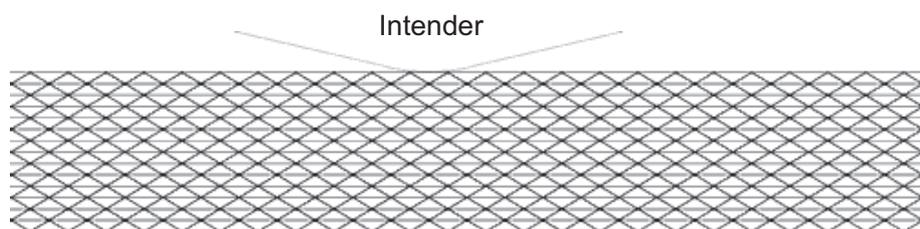
**Figure 5:** Regular 2D AFEM mesh with nano-indenter tip
