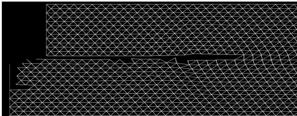
**Figure 7:** Atomic layer delamination simulated by deactivation of inter-atomic bonds
