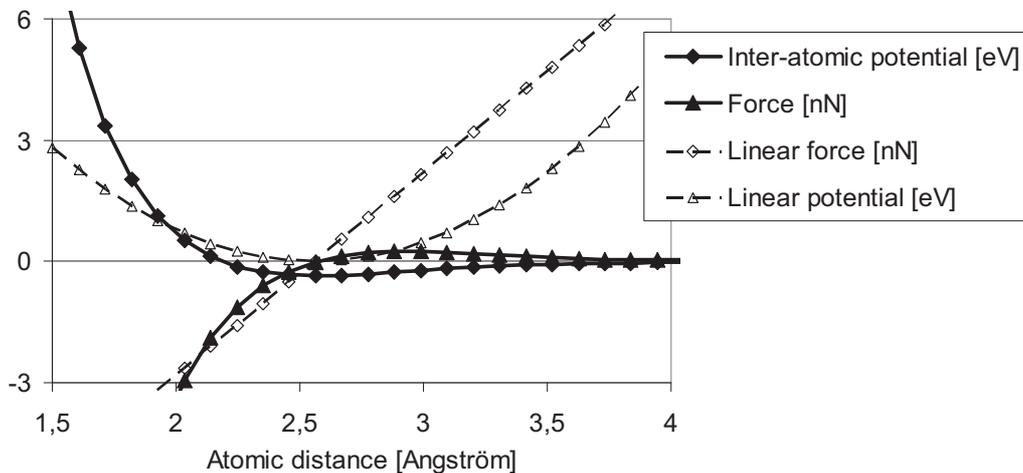
**Figure 4:** Inter-atomic potential of Al-Ni and derived non-linear inter-atomic forces (linear behaviour as comparison)
