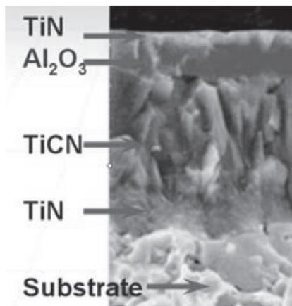
**Figure 1:** Typical multilayer surface system of cutting tool coatings [2]
