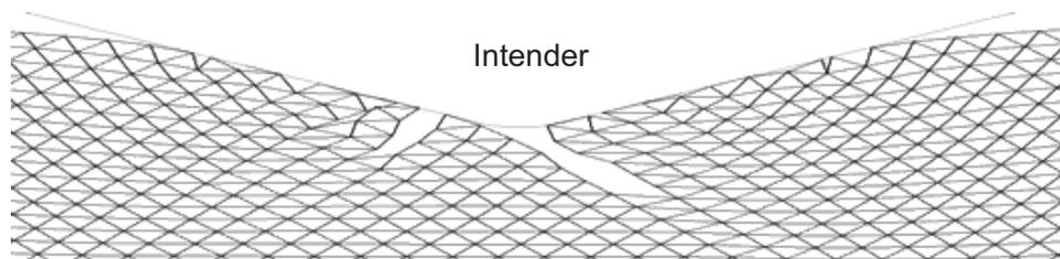
**Figure 6:** Nano-crack initiation simulated by deactivation of inter-atomic bonds
