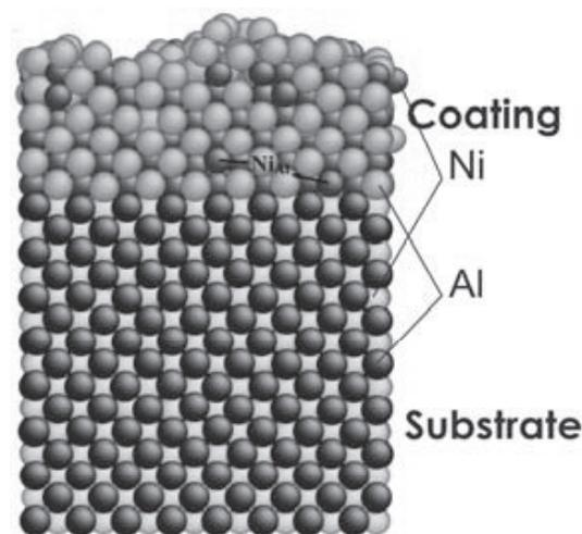
**Figure 2:** Ni-Al Molecular Dynamics simulation
