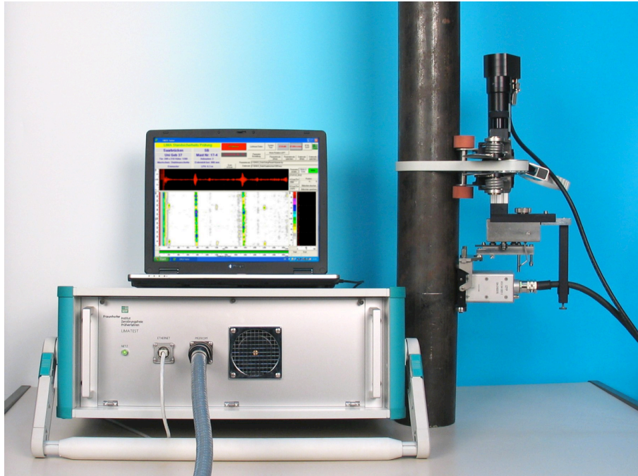
Figure 1. Inspection system for light poles LIMAtest
