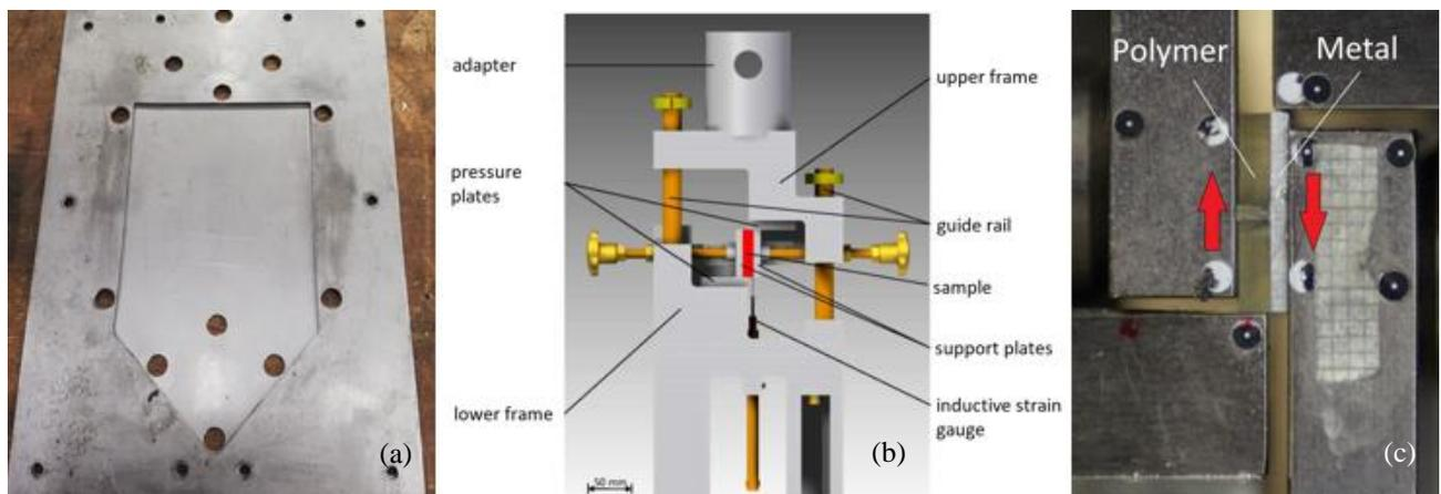
**Figure 1:** (a) Insertion tool [7], (b) testing device of the shear strength test [5] and (c) a mounted test sample.
