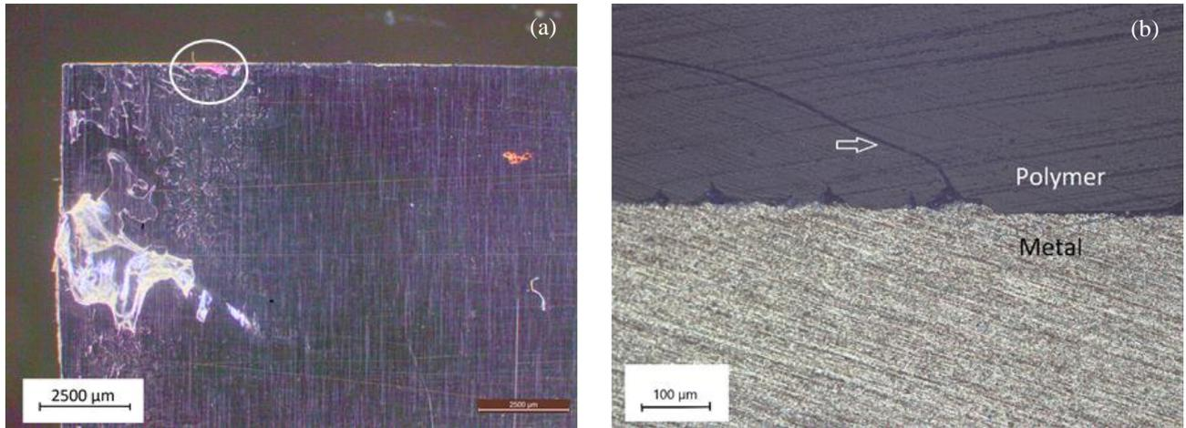
**Figure 4:** (a) Macroscopic analysis of a shear edge sample with polymer arrears in the white circle, (b) microscopic analysis of the interface with a crack structure inside the polymer like a drop-shaped structure [7].
