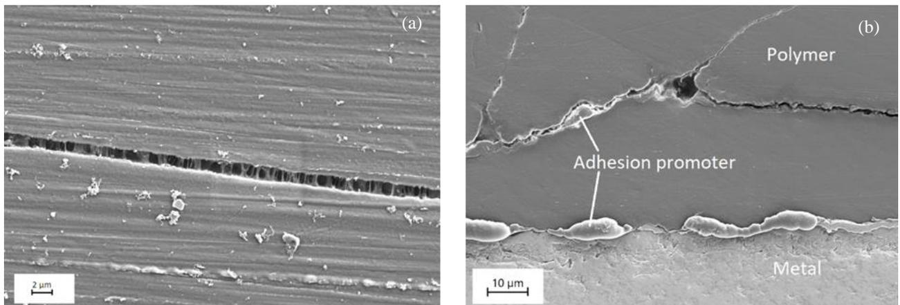
**Figure 5:** (a) Scanning electron microscope analysis of a fissure, (b) the material transition [7].
