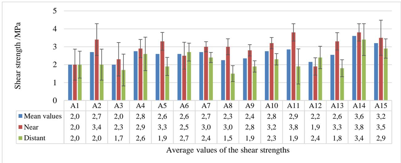
**Figure 2:** Shear strength of different Grilamid TR60 samples, about the hole part (mean values) and near according to further away from the sprue.
