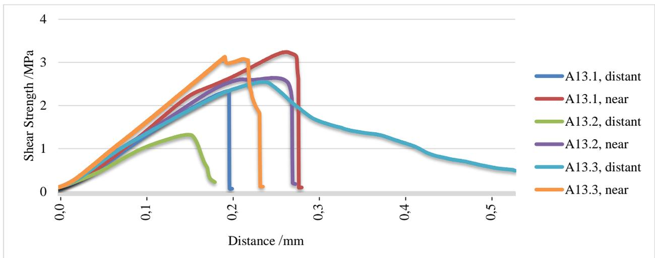
**Figure 3:** Force-displacement-curve after the shear edge test of three samples (Grilamid TR60) with following parameters, mould temperature 60 °C, holding pressure 650 bar and melting temperature 320 °C.
