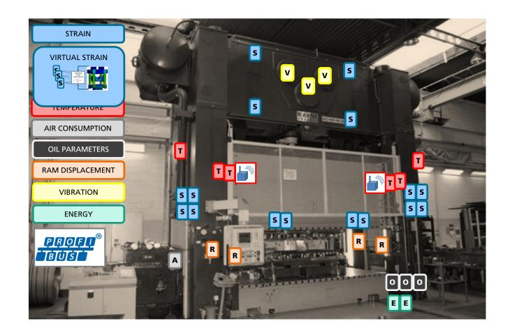
Test example: Artificial intelligence (AI): Model reduction and development of Virtual Sensory by artificial neural networks (ANN)
