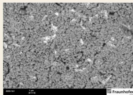
SEM image of the catalytic foam (inlet) after preparation (Ni including segment). SEM image of the catalytic foam (outlet) after preparation (Ir including segment).
