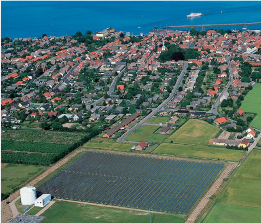
Solar District Heating, Marstal, Denmark collector area 17,000 m 2
