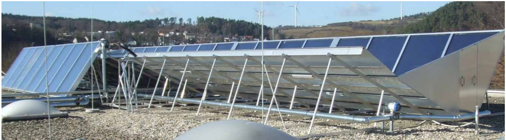
Reference flat-plate collectors (glass-foil, front) and newly developed RefleC-collectors (back)
