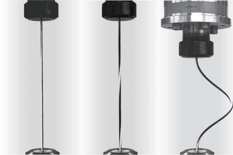
Figure 5: Experimental procedure of multiaxial experiment: A straight specimen is clamped (left), the upper clamp is rotated by  $4\pi$  (middle) and afterwards moved down by 60 mm (right).
